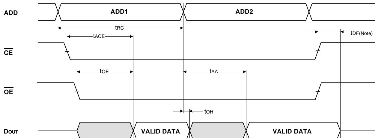
NOTE :  $t_{DF}$  is defined as the time at which the outputs achieve the open circuit condition and is not referenced to  $V_H$  or  $V_L$  level.
