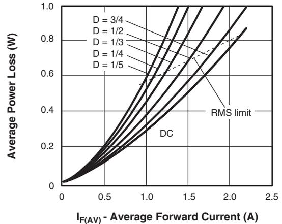
Fig. 5 - Forward Power Loss Characteristics (Per Leg)
