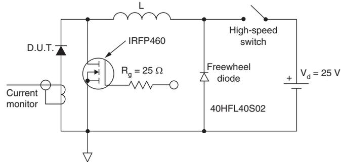
Fig. 7 - Unclamped Inductive Test Circuit
