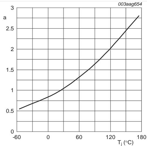
$$a = \frac{R_{DSon}}{R_{DSon(25^\circ\text{C})}}$$
