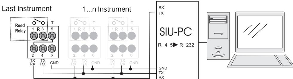
2-wire connection of RS485 serial port + one relay (R). The terminalization must be carried out only on the last instrument of the network
