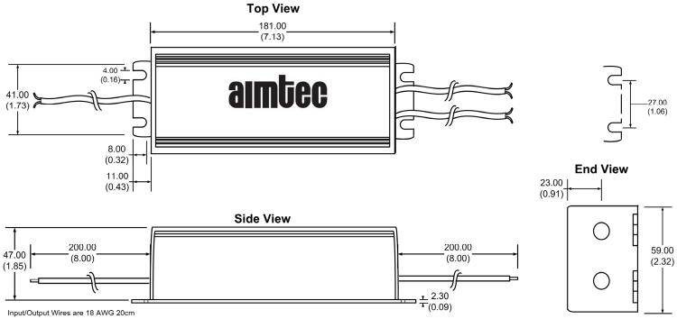
Measurements in Millimeters (inch) Case Tolerance: ±0.5 (±0.02)
