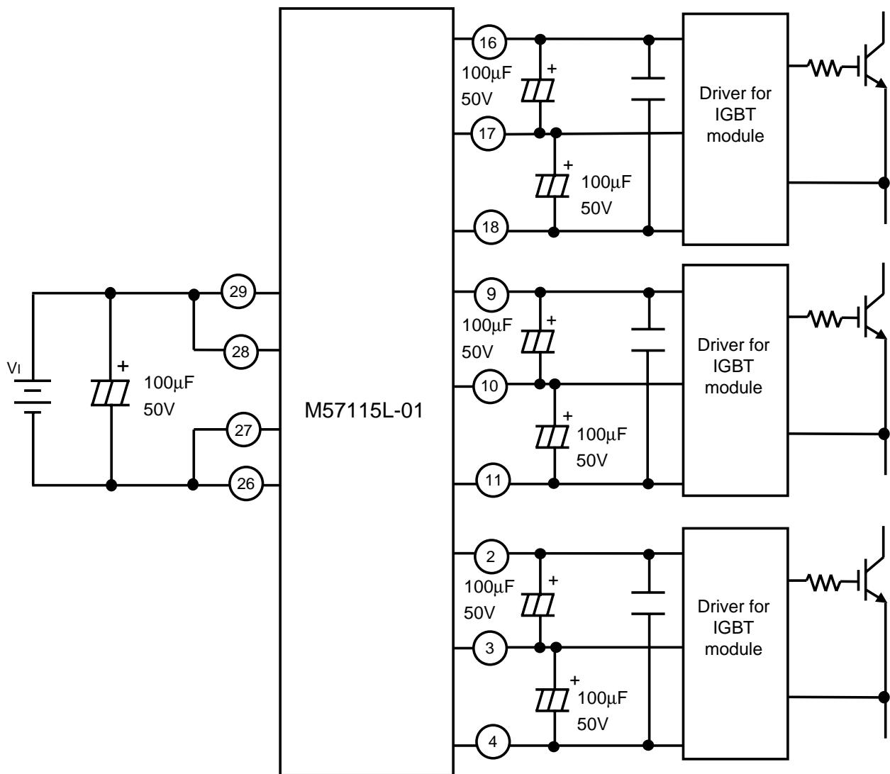
Note) Please select the electrolysis capacitor between each output side terminal (2)-(3), (3)-(4), (9)-(10), and (10)-(11), (16)-(17), and (17)-(18) in consideration of the ripple current of a capacitor etc. with the peak value of gate current.
