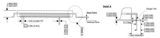
All dimension in mm (inches). Notation is  $\frac{\text{MAX}}{\text{MIN}}$  or typical.
