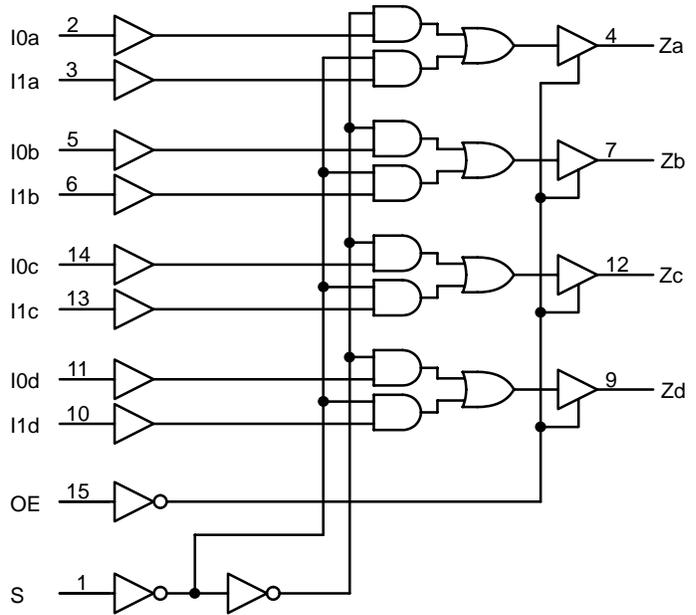
**Figure 2. Logic Diagram**
