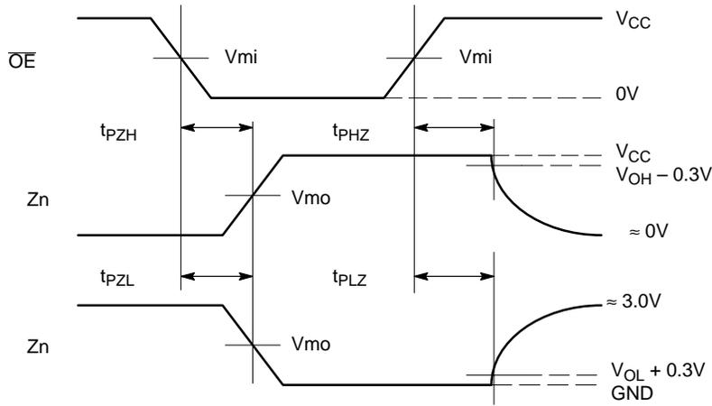
**WAVEFORM 3 – OUTPUT ENABLE AND DISABLE TIMES**
