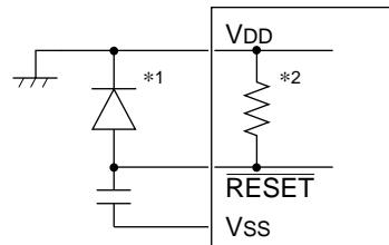
\*1 Because the potential of the RESET terminal not reached VDD level or higher.
