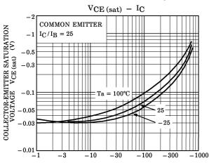
$\begin{array}{cccc} \text{Collector current} & \text{I}_{C} & \text{(mA)} \end{array}$
