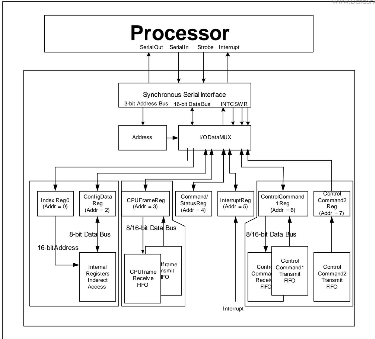
Figure 5 - Overview of the SSI Interface
