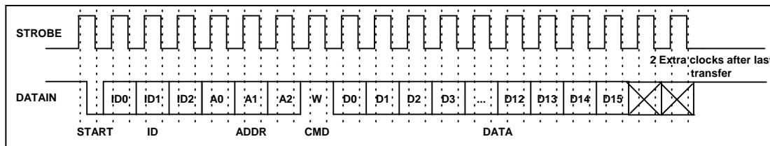
Figure 8 - Serial Interface Write Command Functional Timing
