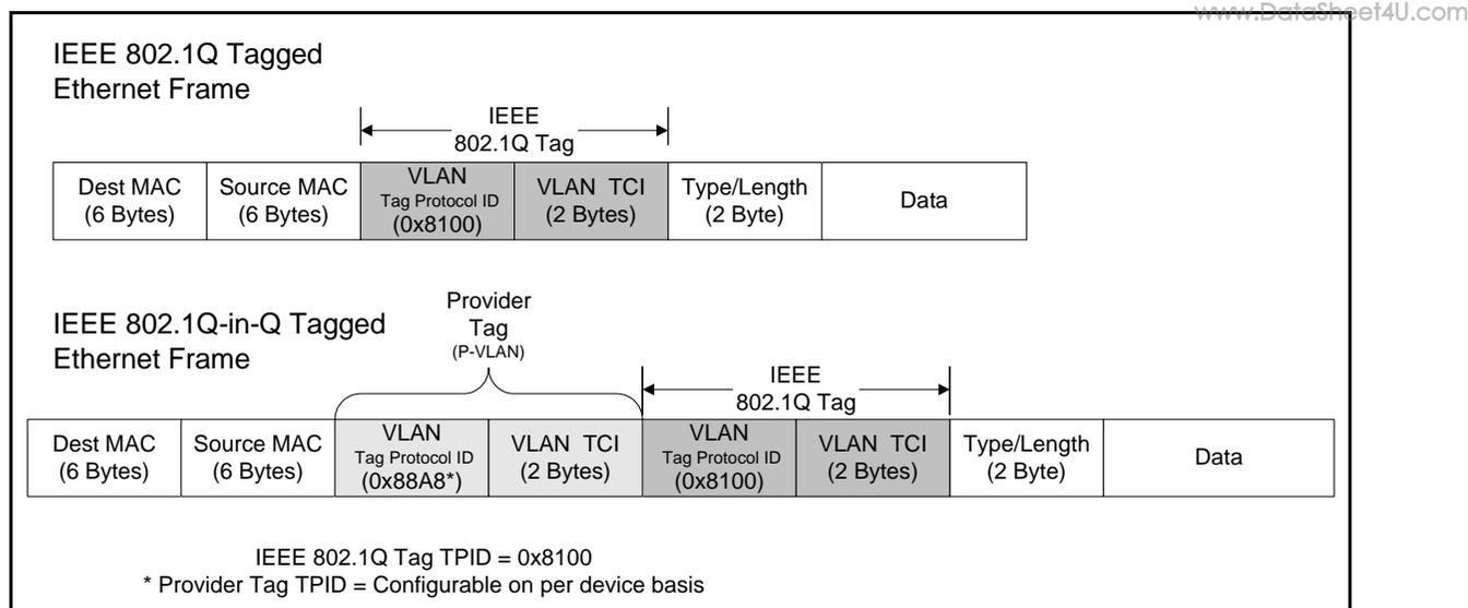
**Figure 11 - Q-in-Q Tagged Ethernet Frame**
