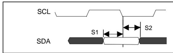
Figure 19 - I<sup>2</sup>C Setup & Hold Timing
