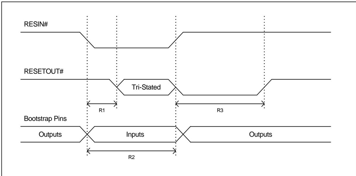
Figure 14 - Typical Reset & Bootstrap Timing Diagram
