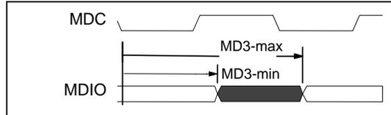
Figure 32 - MDIO Output Delay Timing
