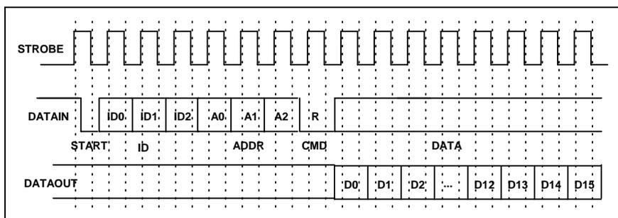
Figure 9 - Serial Interface Read Command Functional Timing
