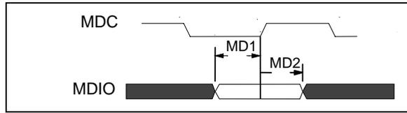
Figure 31 - MDIO Setup & Hold Timing
