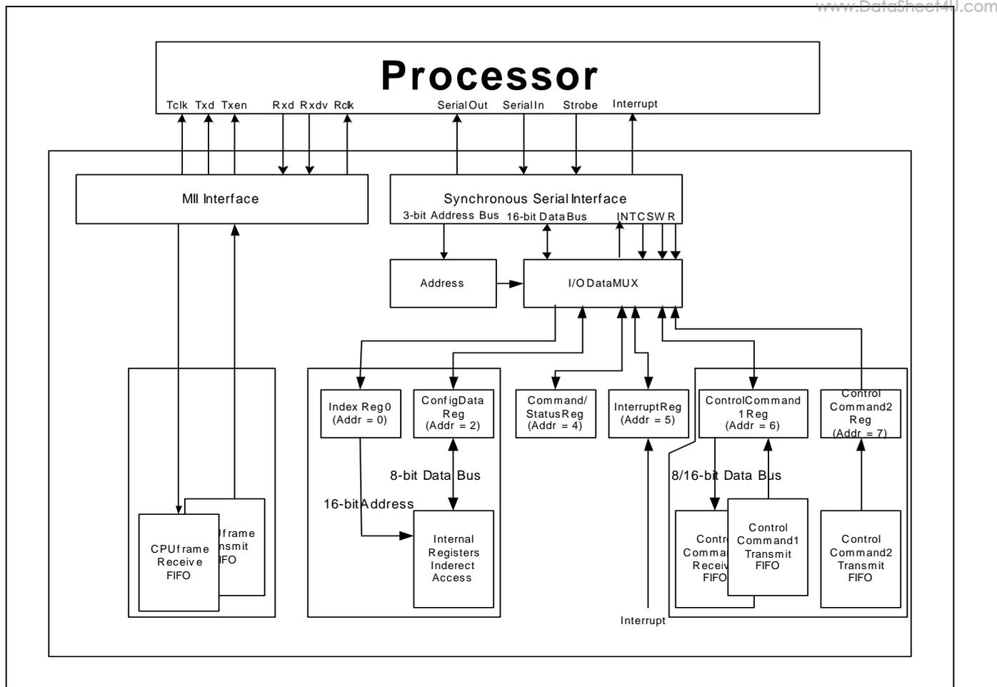
Figure 6 - Overview of the SSI+MII Interface
