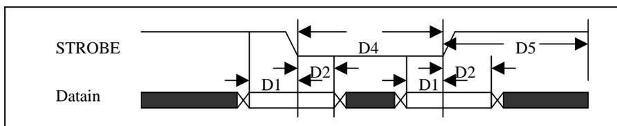
Figure 17 - SSI Setup & Hold Timing
