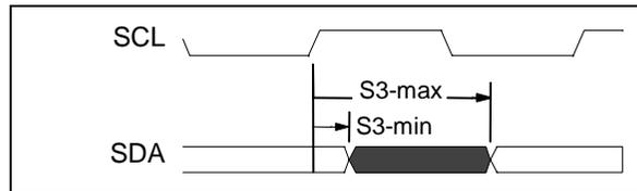
Figure 20 - I<sup>2</sup>C Output Delay Timing
