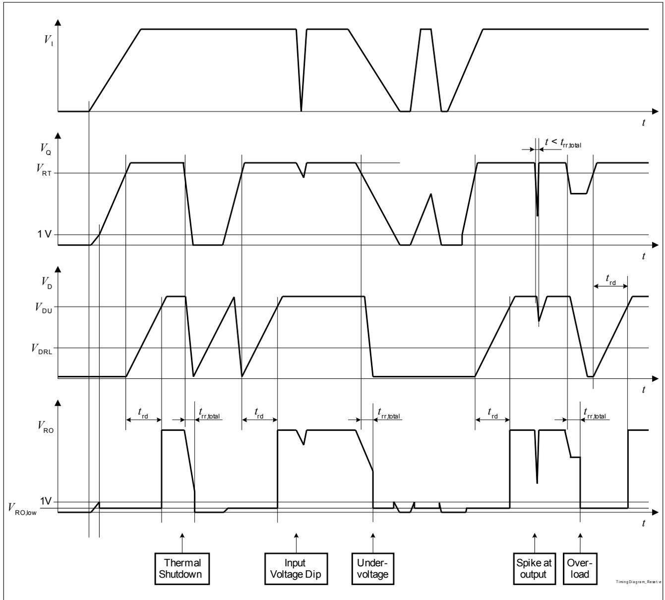
Figure 6 Timing Diagram Reset
