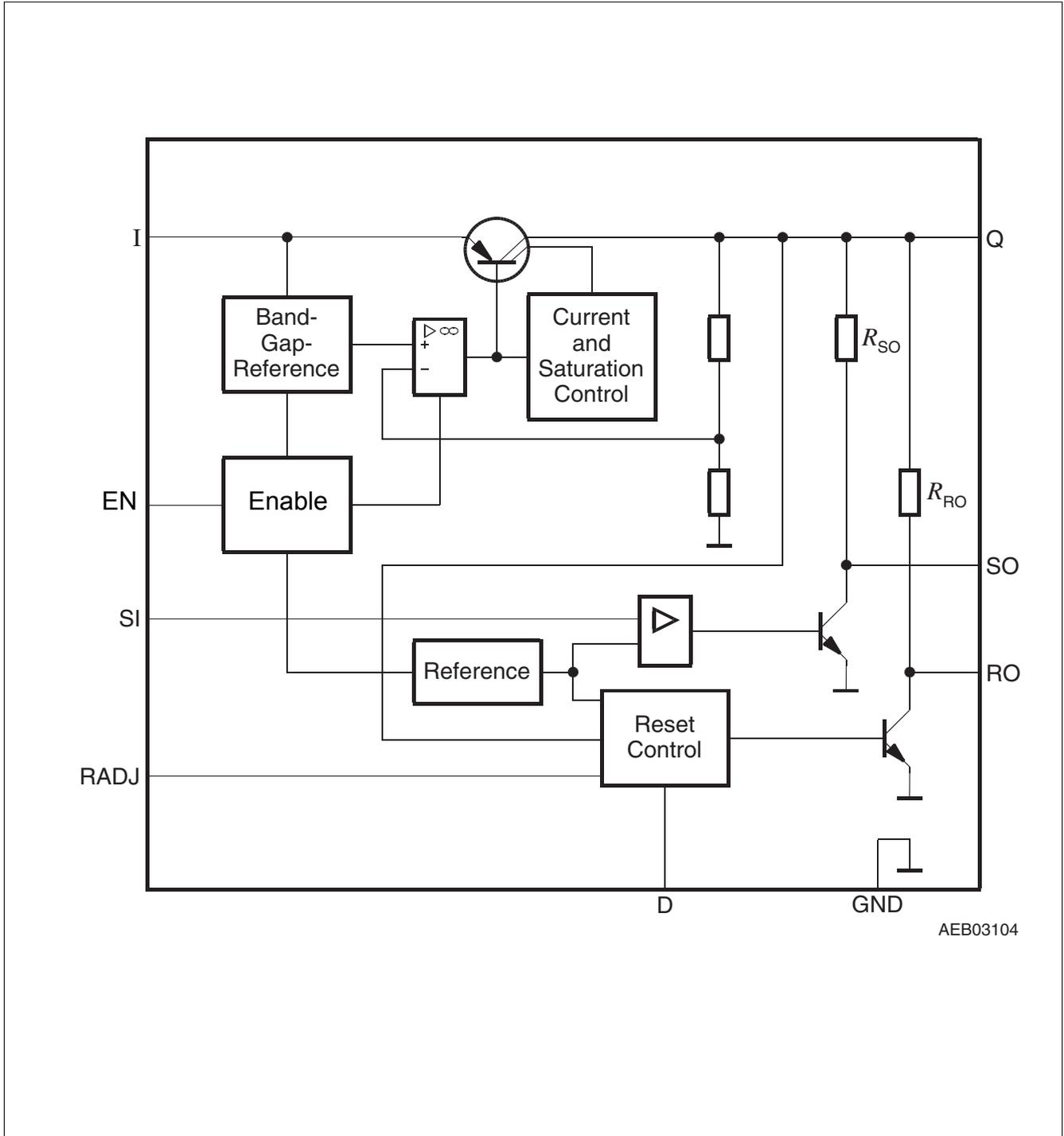
Figure 1 Block Diagram
