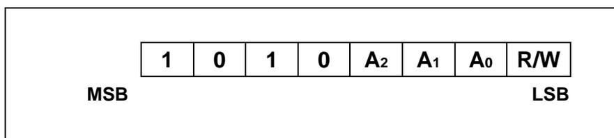
Figure 7 · Device Address
