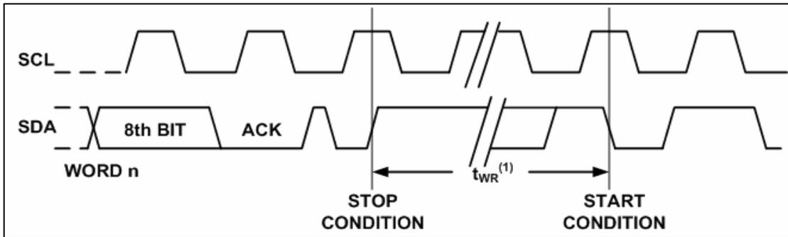
Figure 3. SCL: Serial Clock, SDA: Serial Data I/O
