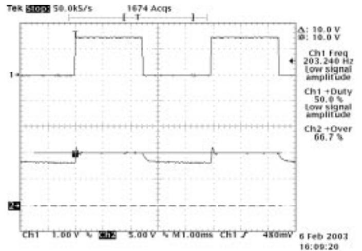
Channel 1 is the Enable waveform
