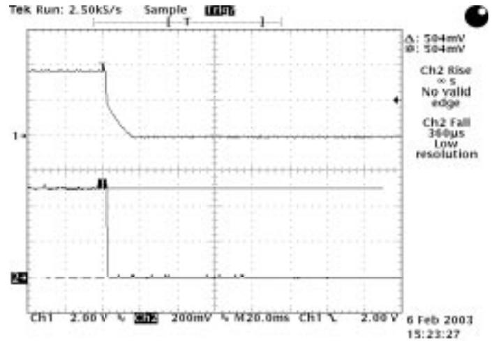
Channel 1 Supply Voltage turns off
