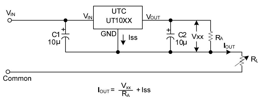
$$I_{OUT} = \frac{V_{xx}}{R_A} + I_{ss}$$
