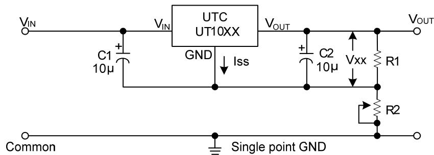
$$V_{OUT} = V_{xx}(1 + \frac{R2}{R1}) + I_{ss}R2$$
