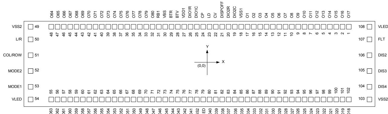
Chip Size: 7960µm x 1470µm
