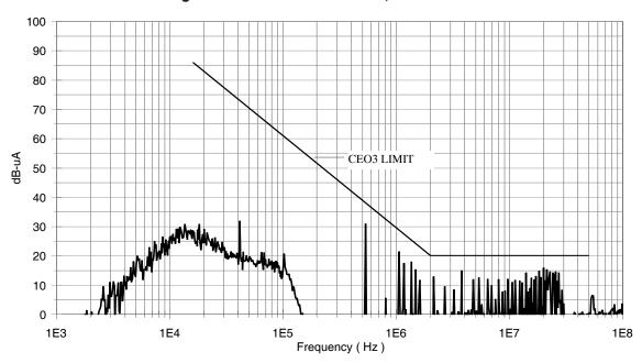
Figure 3. Conducted Emissions, Return Lead
