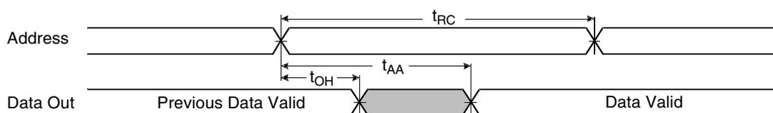
**Note:** CE1#s = OE# =  $V_{IL}$ , CE2s = WE# =  $V_{IH}$ , UB#s and/or LB#s =  $V_{IL}$
