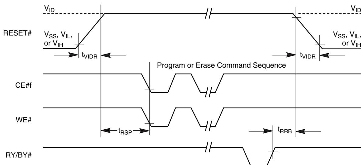
**Figure 25. Temporary Sector/Sector Block Unprotect Timing Diagram**
