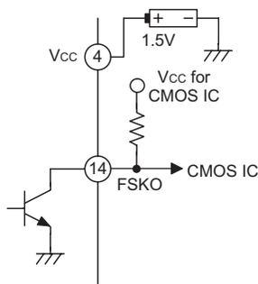
**Quick charge-discharge circuit**
