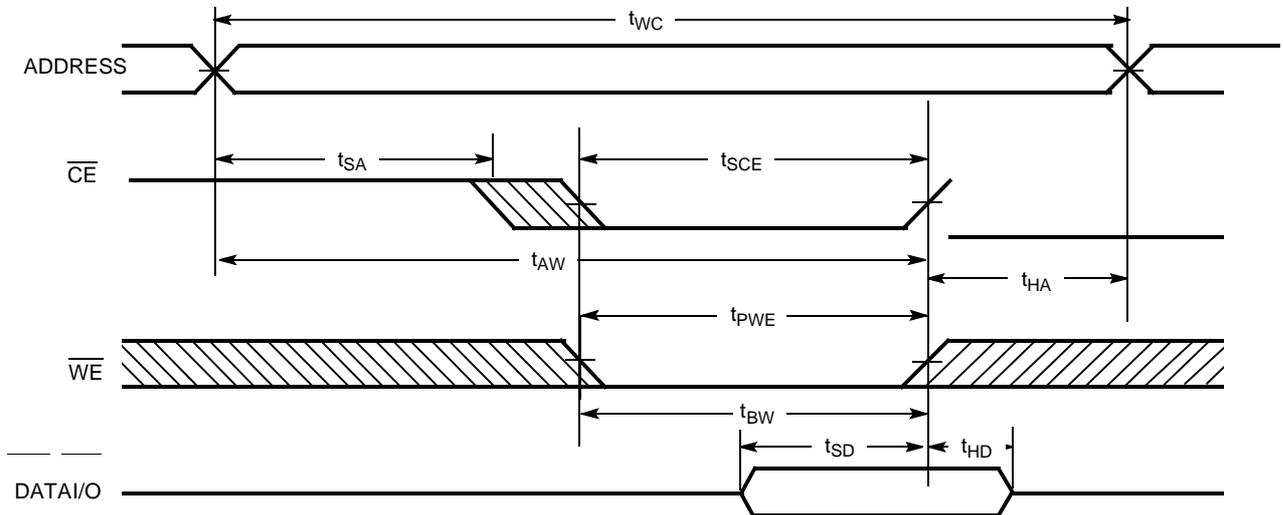
Write Cycle No. 2 ( $\overline{WE}$  Controlled,  $\overline{OE}$  LOW)<sup>[16, 17, 18]</sup>
