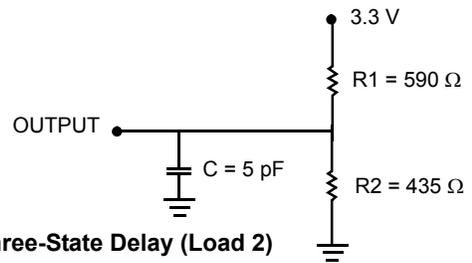
(b) Three-State Delay (Load 2)
