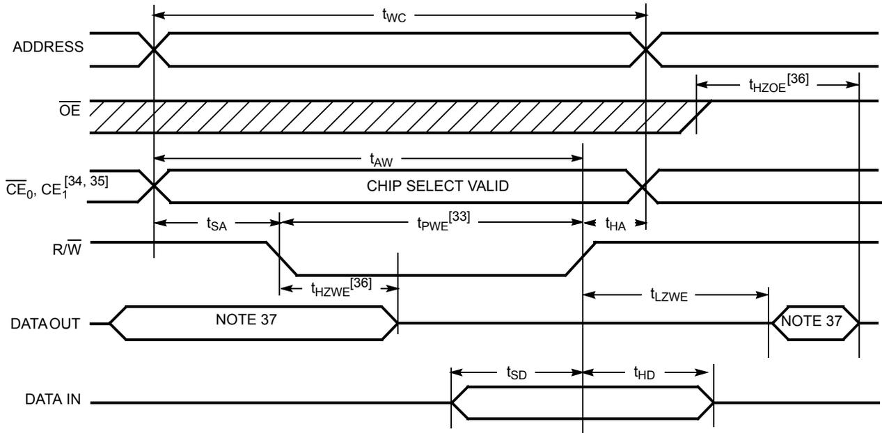
Write Cycle No. 2: CE Controlled Timing<sup>[30, 31, 32, 38]</sup>
