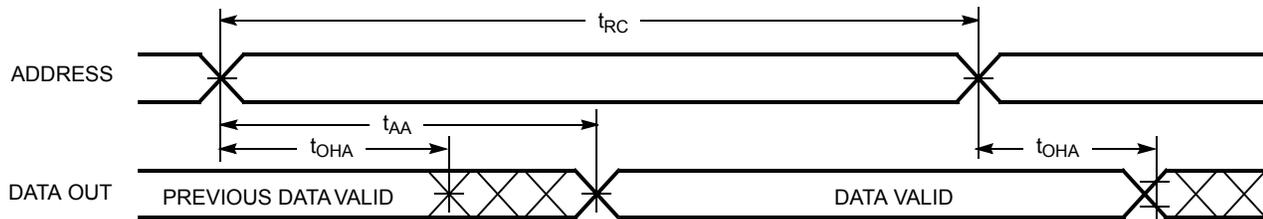
**Read Cycle No. 2 (Either Port  $\overline{CE}/\overline{OE}$  Access)**<sup>[25, 28, 29]</sup>
