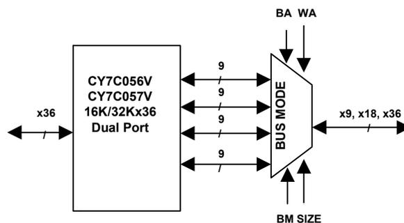
The bus match select (BM) pin works with bus size select (SIZE) to select bus width (long-word, word, or byte) for the right port of the dual-port device. The data sequencing arrangement is selected using the word address (WA) and byte address (BA) input pins. A logic "0" applied to both the bus match select (BM)
