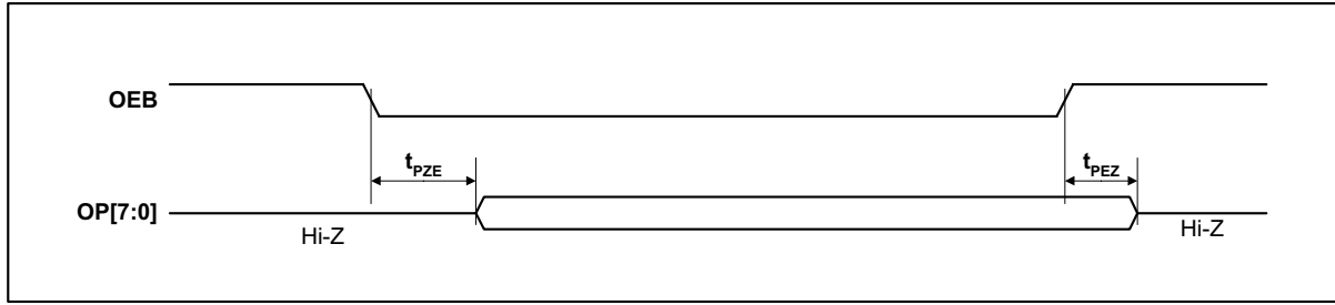
Figure 3 Output Data Enable Timing
