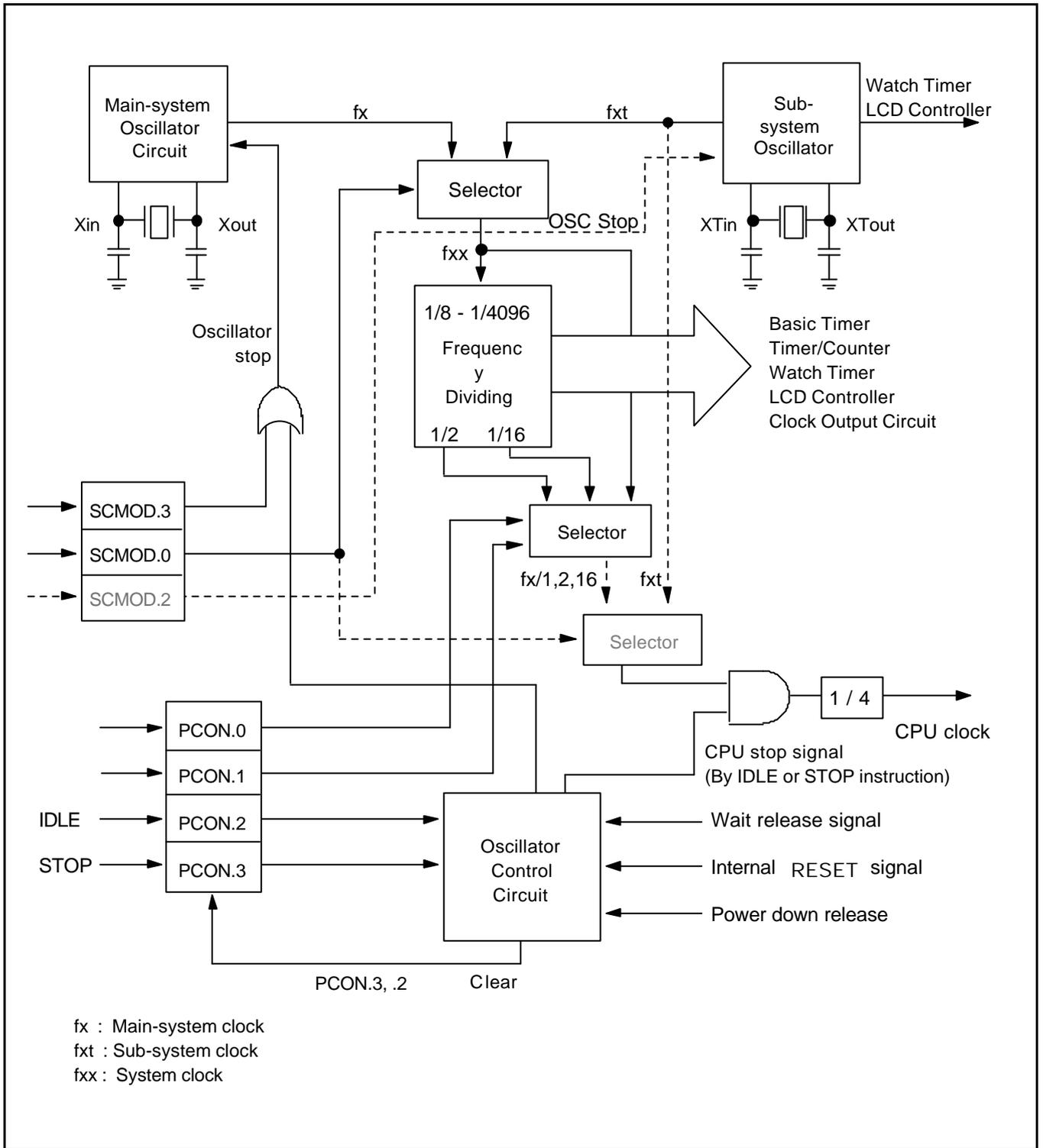
Figure 6-1. Clock Circuit Diagram
