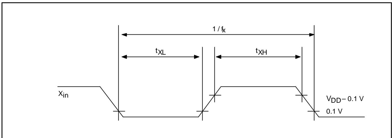
Figure 13-5. Clock Timing Measurement at  $X_{in}$
