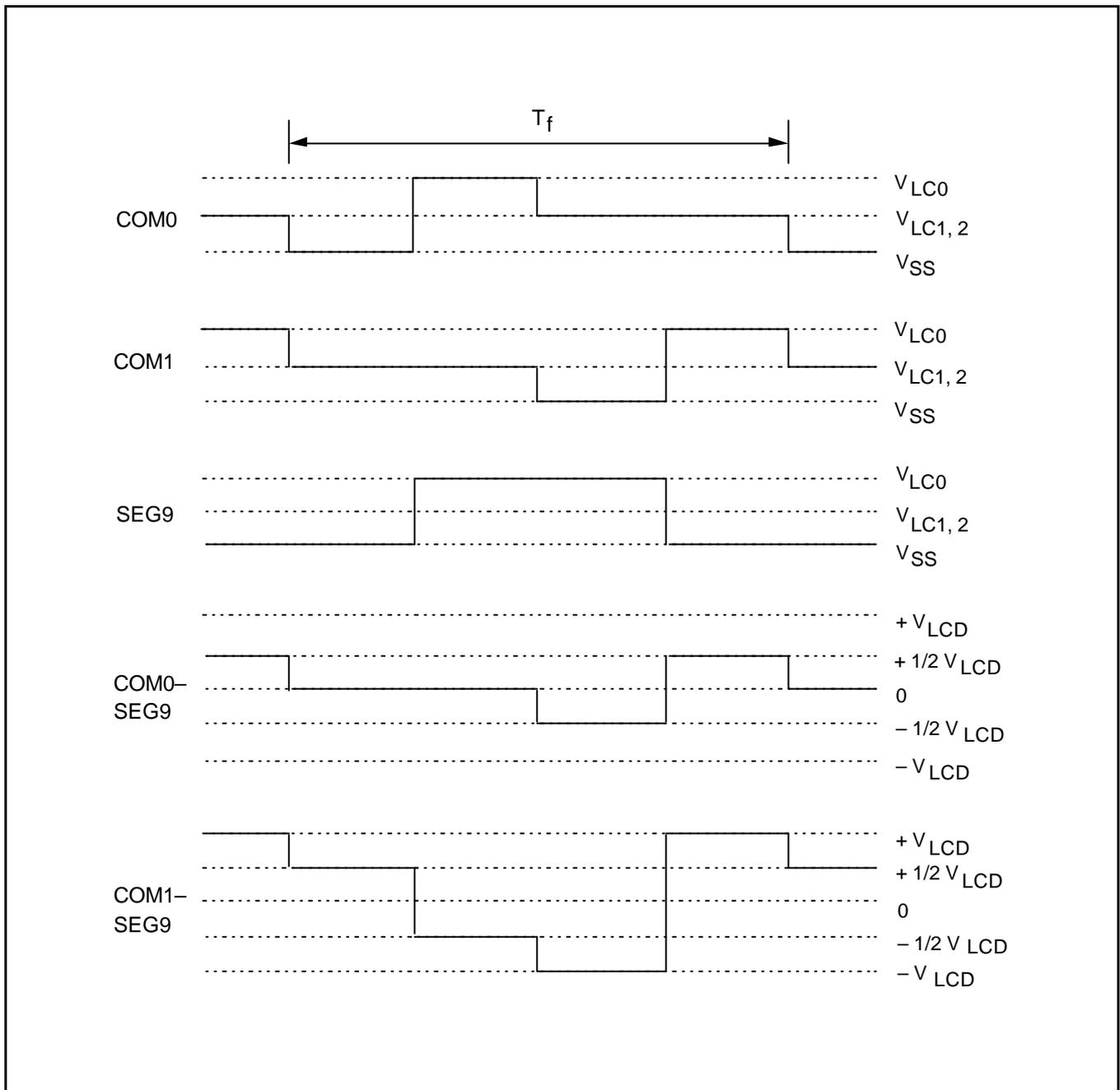
Figure 12-7. LCD Signal Waveforms at 1/2 Duty, 1/2 Bias
