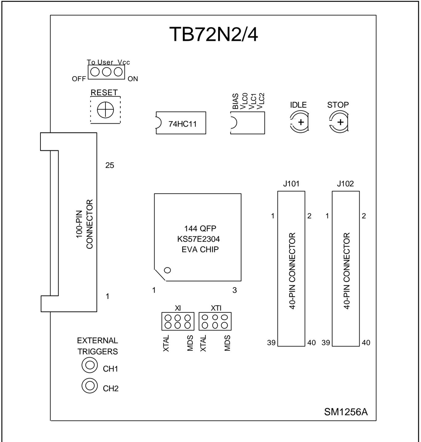
Figure 16-2. TB72N2/4 Target Board Configuration
