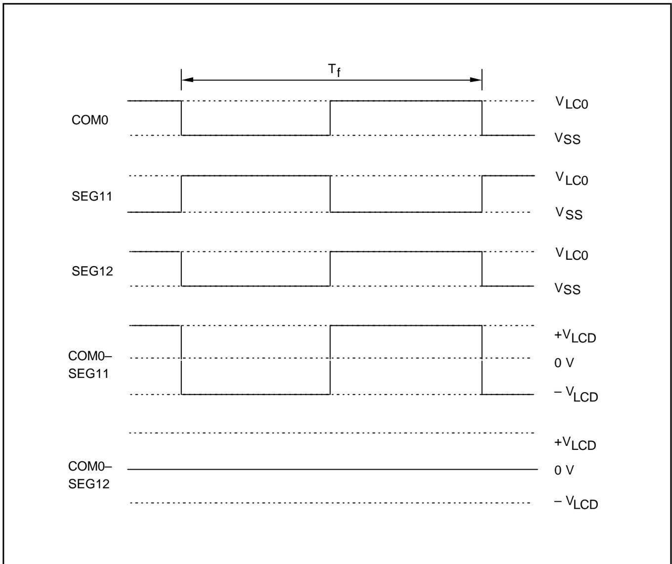
Figure 12-5. LCD Signal Waveforms in Static Mode
