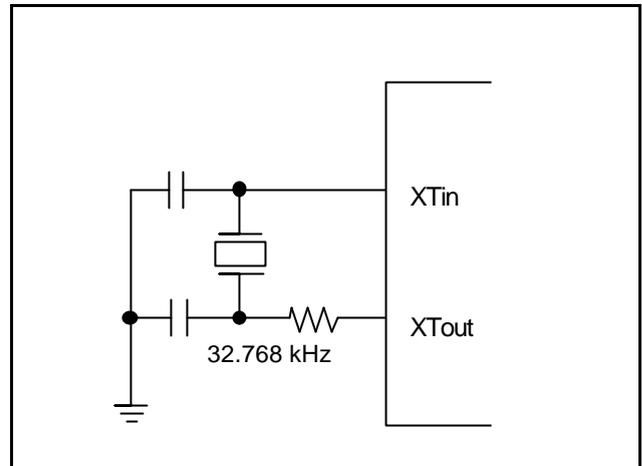
Figure 6-5. Crystal/Ceramic Oscillator
