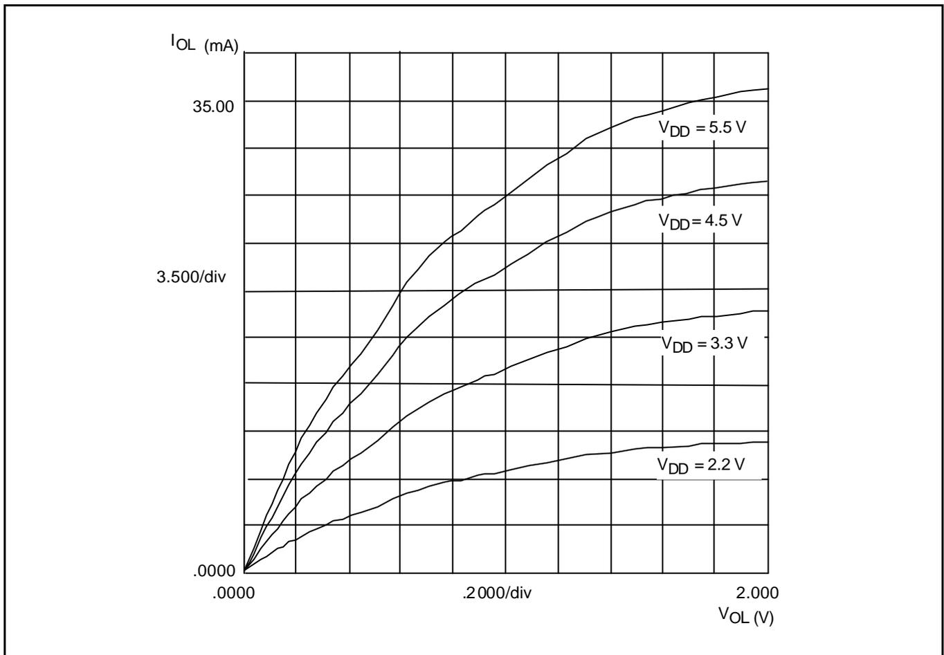
Figure 15-3. Port 2  $I_{OL}$  vs  $V_{OL}$  Curve
