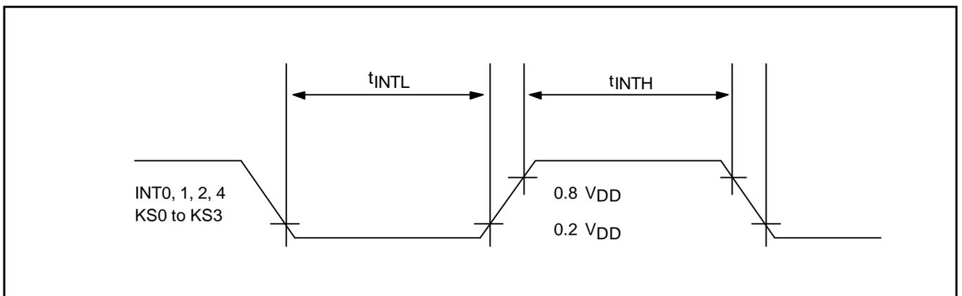
Figure 13-9. Input Timing for External Interrupts and Quasi-Interrupts
