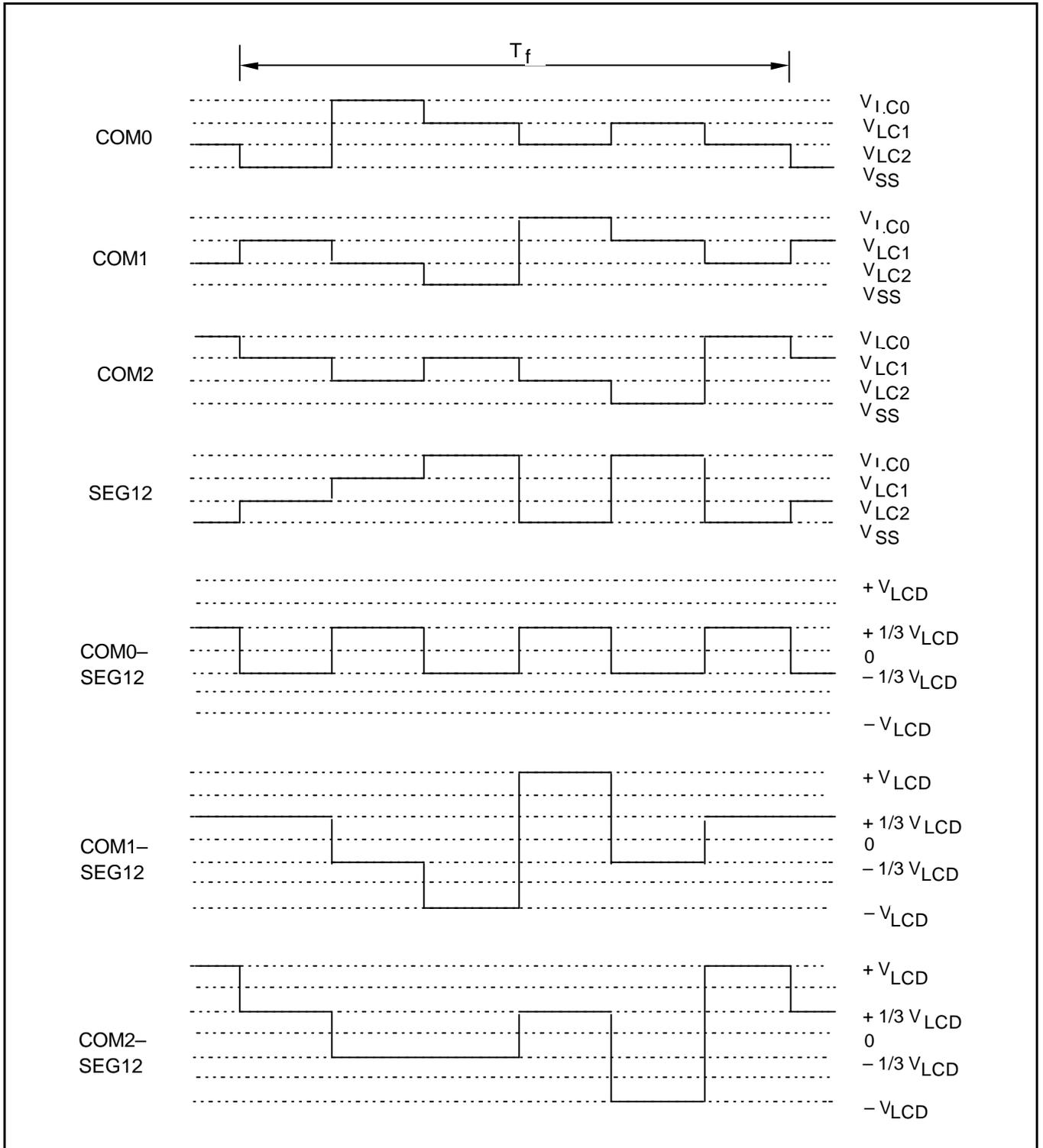
Figure 12-10. LCD Signal Waveforms at 1/3 Duty, 1/3 Bias
