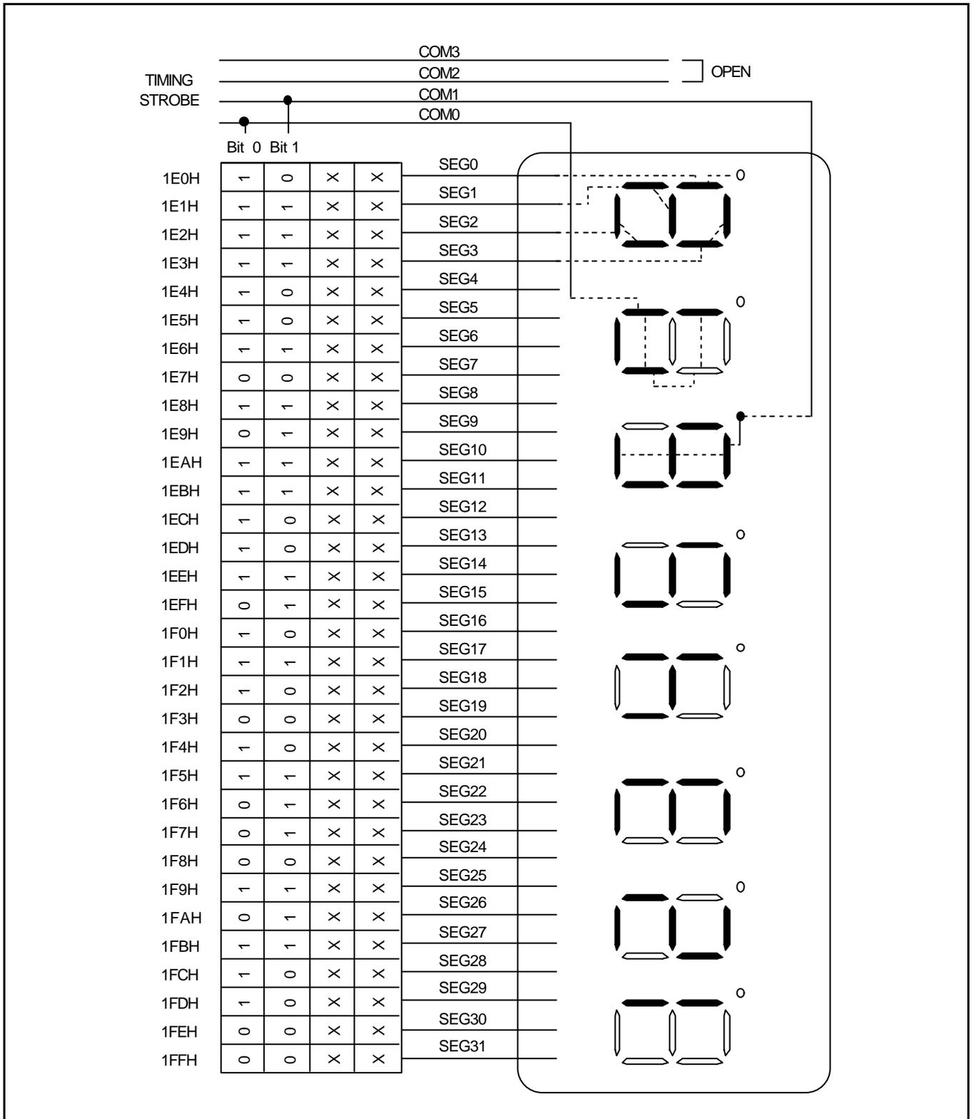
Figure 12-8. LCD Connection Example at 1/2 Duty, 1/2 Bias
