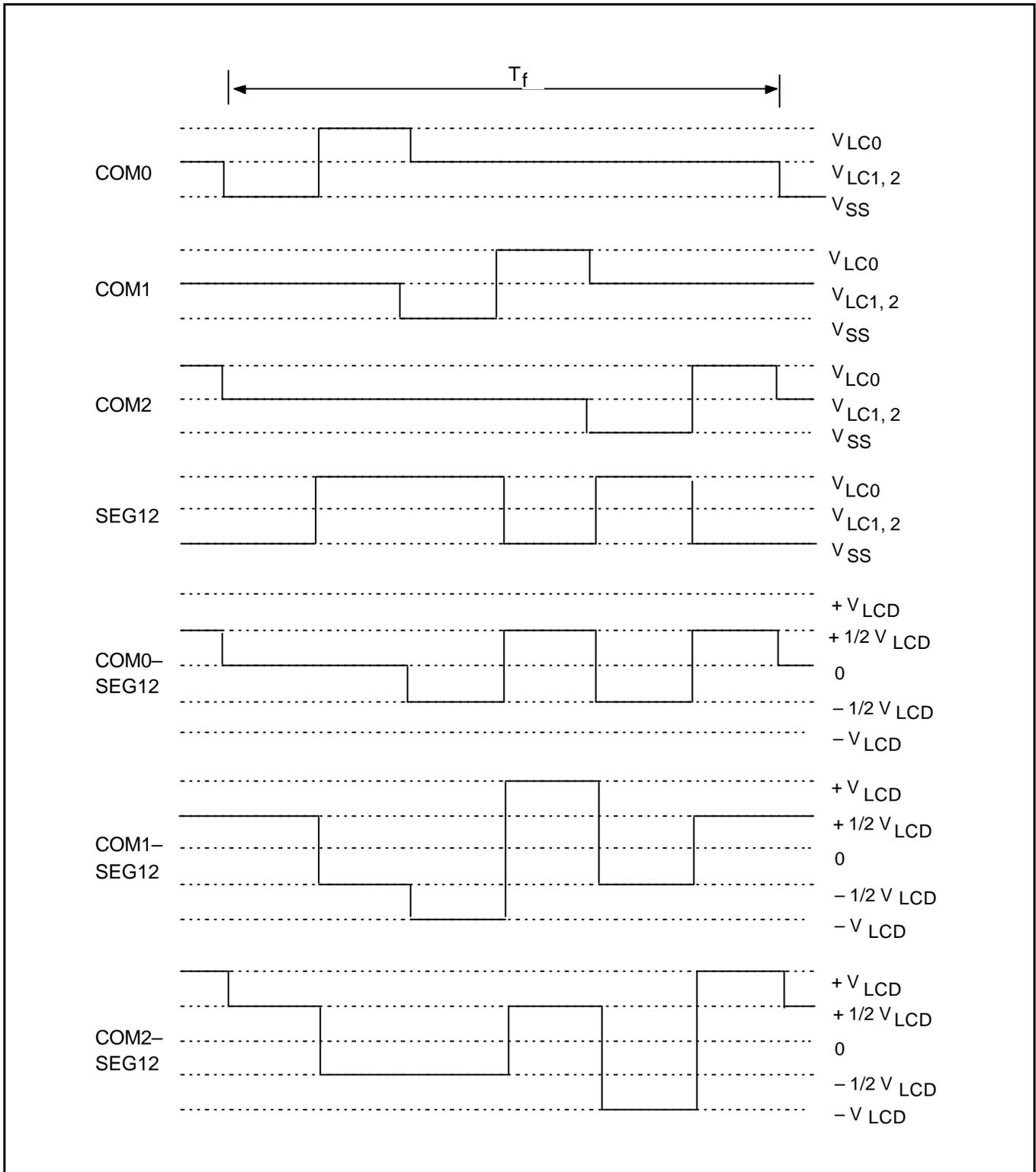
Figure 12-9. LCD Signal Waveforms at 1/3 Duty, 1/2 Bias
