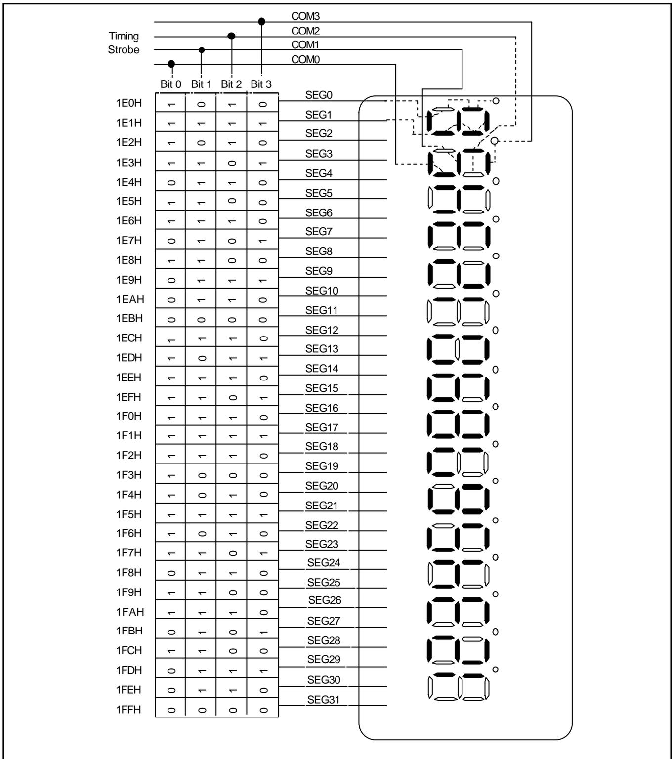
Figure 12-13. LCD Connection Example at 1/4 Duty, 1/3 Bias
