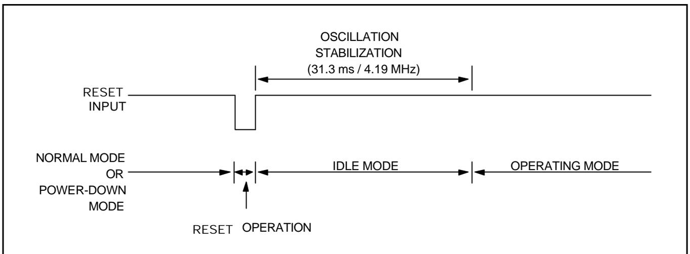
Figure 9-1. Timing for Oscillation Stabilization After RESET
