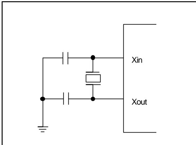
Figure 6-2. Crystal/Ceramic Oscillator
