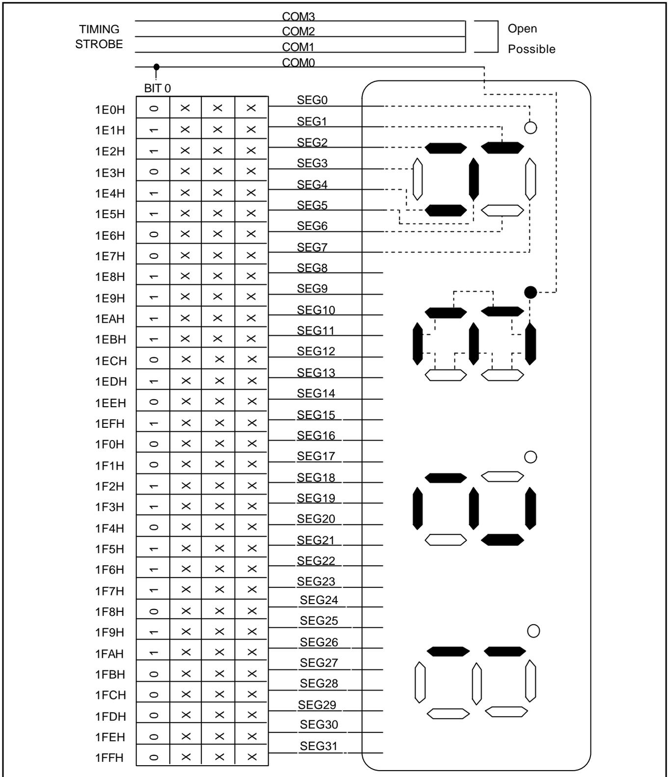
Figure 12-6. LCD Connection Example in Static Mode
