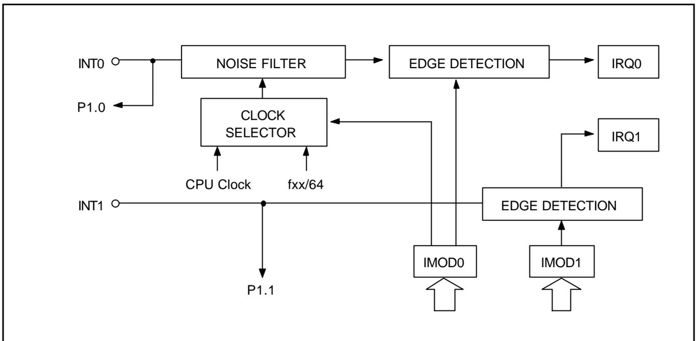
**Figure 7-5. Circuit Diagram for INT0 and INT1 Pins**
