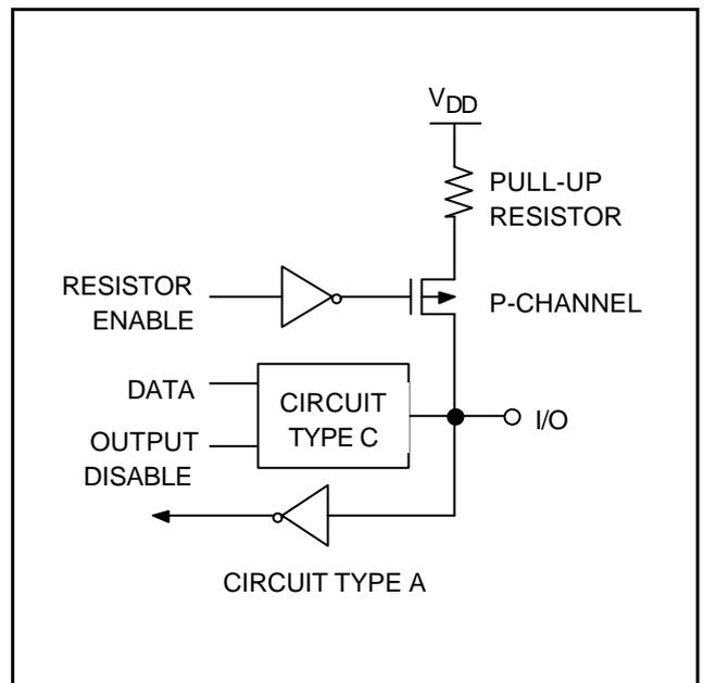
**Figure 1-6. Pin Circuit Type D (P2, P3, and P6)**
