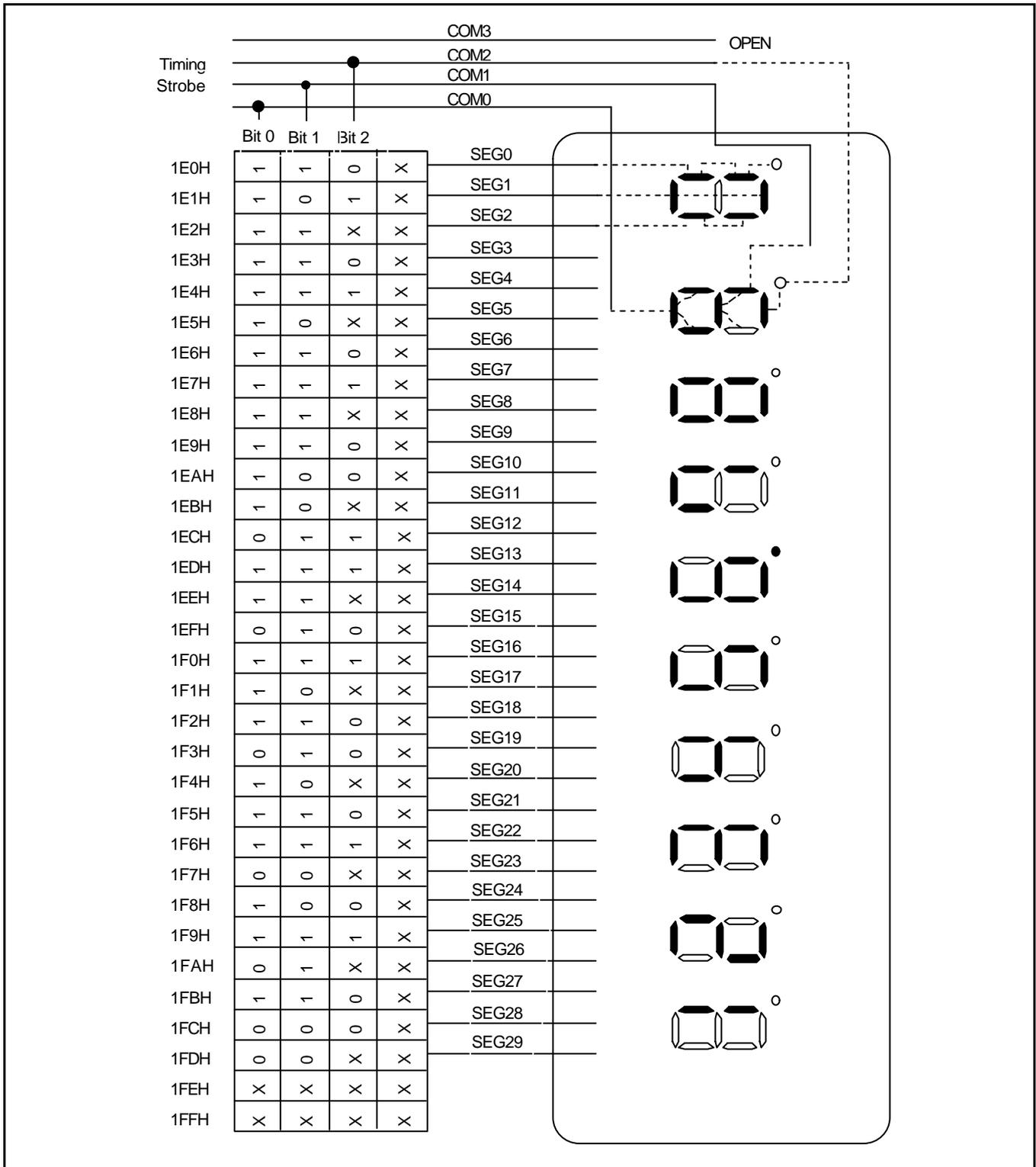
Figure 12-11. LCD Connection Example at 1/3 Duty, 1/3 Bias
