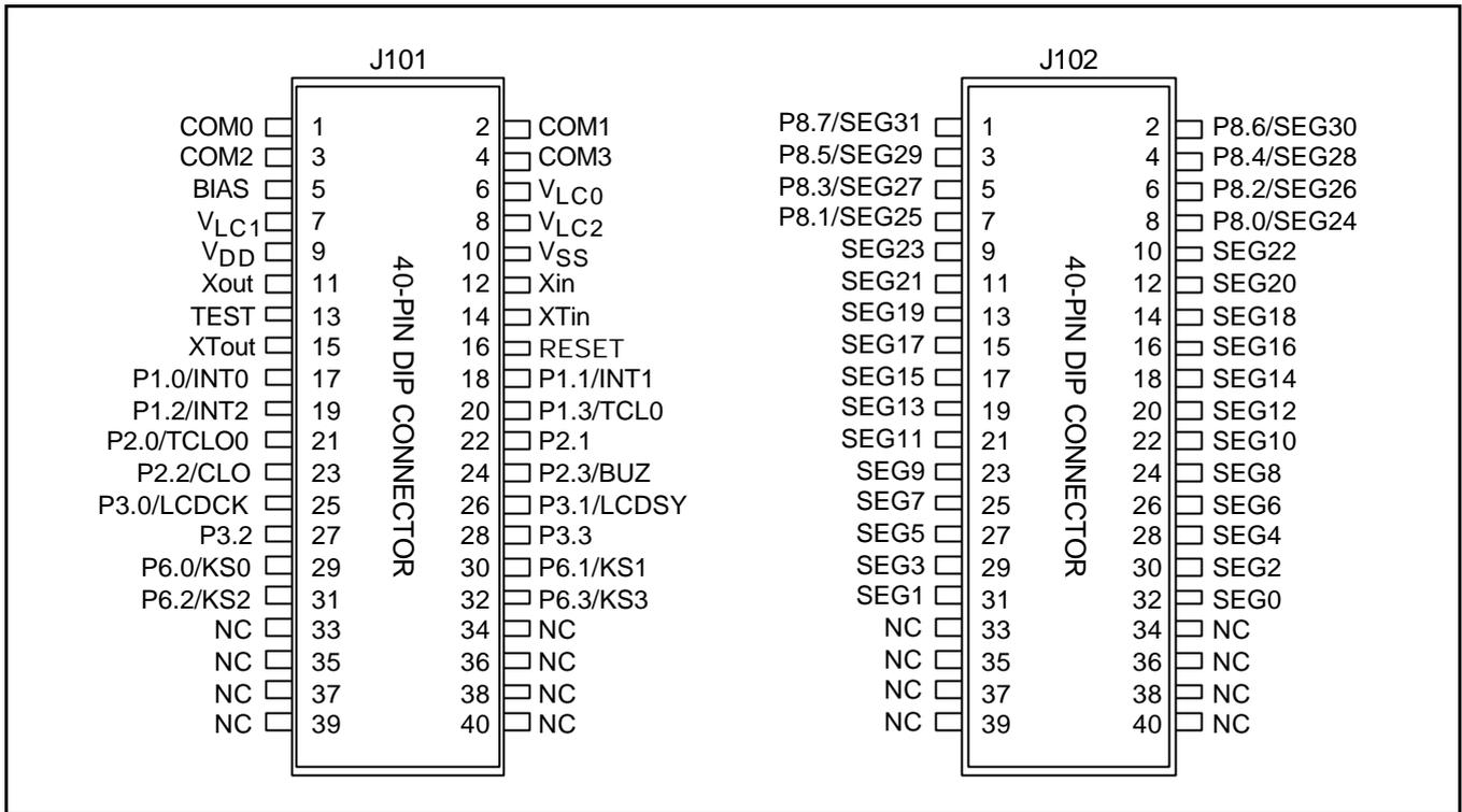
Figure 16-3. 40-Pin Connectors for TB72N2/4
