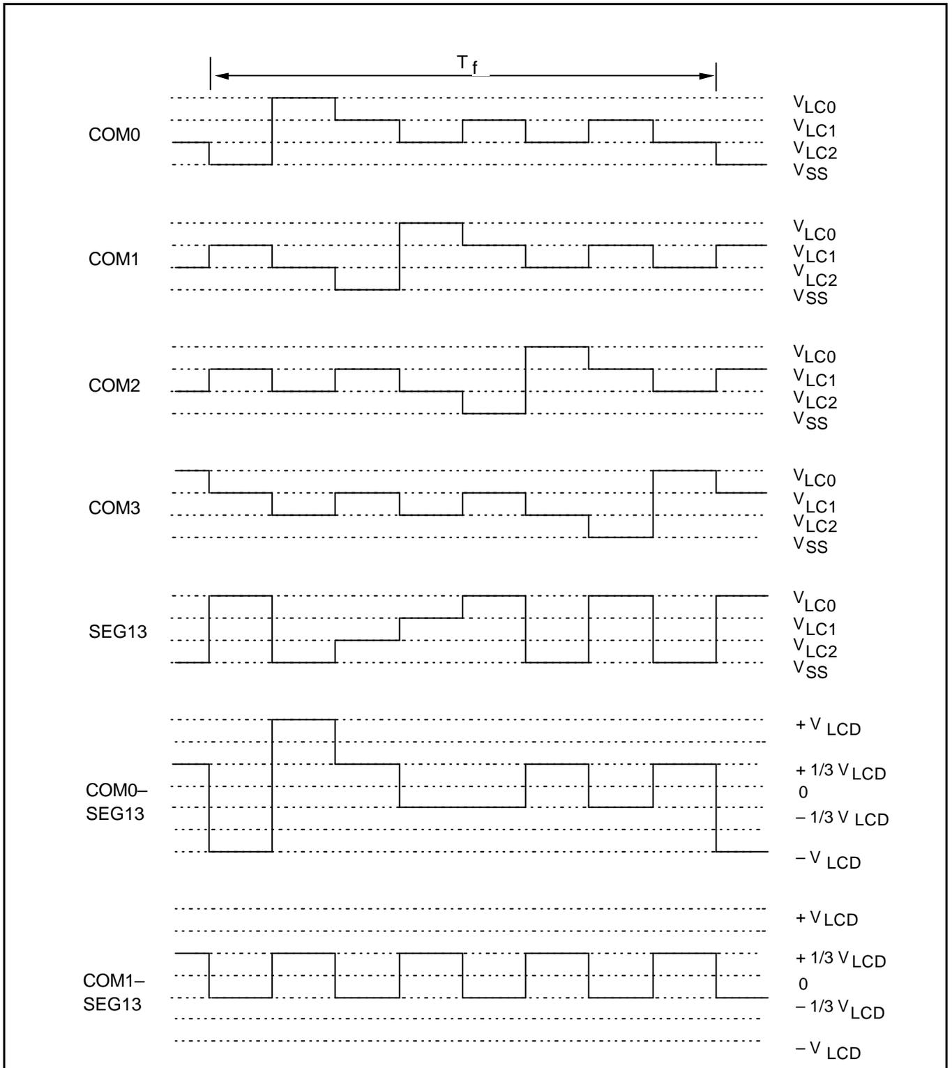
Figure 12-12. LCD Signal Waveforms at 1/4 Duty, 1/3 Bias
