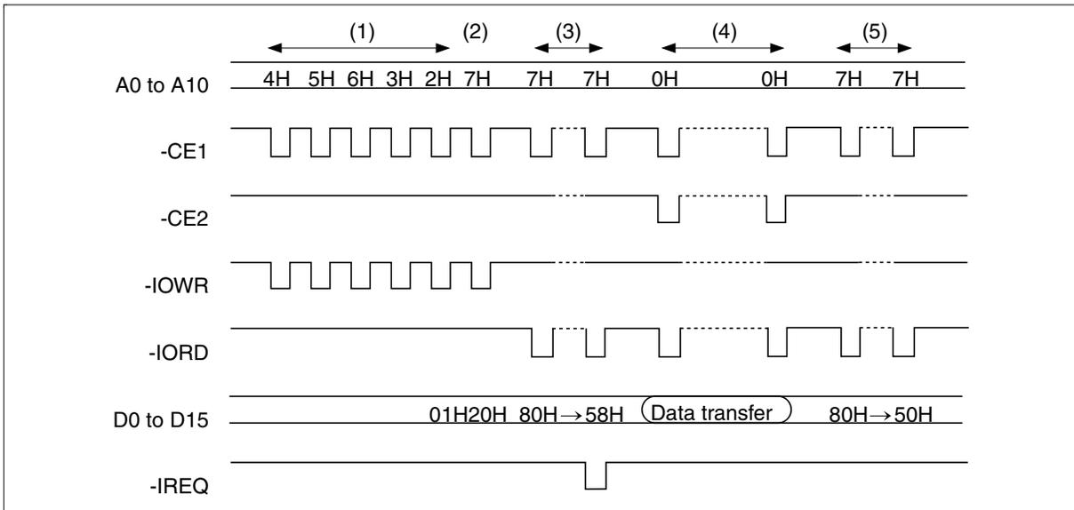
2. Sector write: 1 sector write procedure after the card configured I/O interface is shown as follows.
