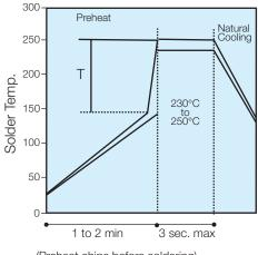
(Preheat chips before soldering) T/maximum 150°C
