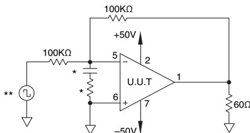
\* These components are used to stabilize device due to poor high frequency characteristics of burn in board.
