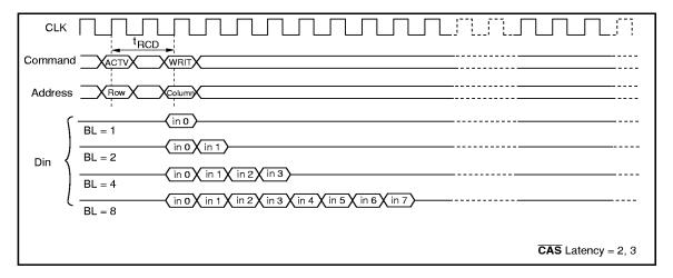
**2. Single write:** A single write operation is enabled by setting OPCODE (A9, A8) to (1, 0). In a single write operation, data is only written to the column address (AY0 to AY8; HM5225165B, AY0 to AY9; HM5225805B, AY0 to AY9, AY11; HM5225405B) and the bank select address (BA0/BA1) specified by the write command set cycle without regard to the burst length setting. (The latency of data input is 0 clock).
