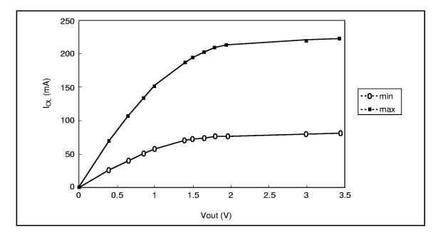
Output High Current (I $_{OH}$ ) (Ta = 0 to 70°C, V $_{CC}$ , V $_{CC}$ Q = 3.0 V to 3.45 V, V $_{SS}$ , V $_{SS}$ Q = 0 V)
