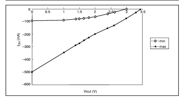
DC Characteristics (Ta = 0 to 70°C,  $V_{CC},\,V_{CC}Q$  = 3.3 V  $\pm$  0.3 V,  $V_{SS},\,V_{SS}Q$  = 0 V) (HM5225165B)
