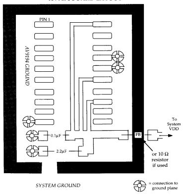
This is the recommended layout for the AV9194. Shown are the power connections and the ground plane.
