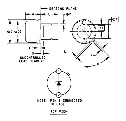
FIGURE 1. Case outline dimensions and terminal connections.
