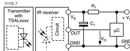
The external components  $R_1$  and  $C_1$  are optional to improve the robustness against electrical overstress (typical values are  $R_1 = 100 \Omega$ ,  $C_1 = 0.1 \mu F$ ). The output voltage  $V_o$  should not be pulled down to a level below 1 V by the external circuit. The capacitive load at the output should be less than 2 nF.
