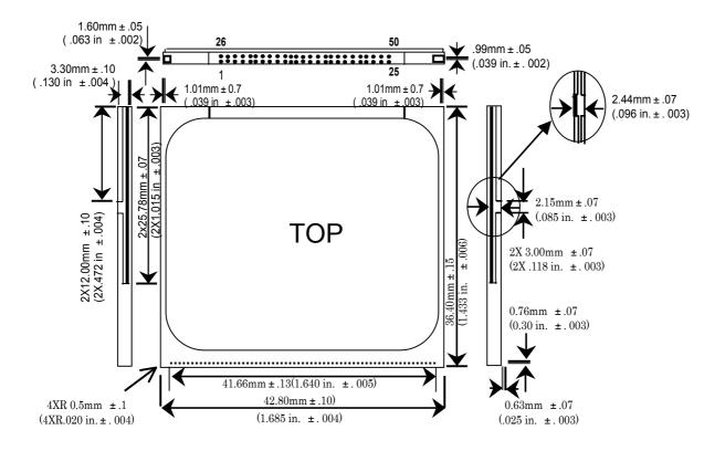
Note: The optional notched configuration was shown in the CF Specification Rev.1.0. In Specification Rev. 1.2. the notch was removed for ease of tooling. This optional configuration can be used but it is not recommended.
