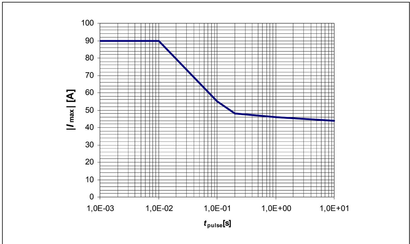
**Figure 4** BTN7975B Maximum Single Pulse Current ( $T_C < 85^\circ\text{C}$ )
