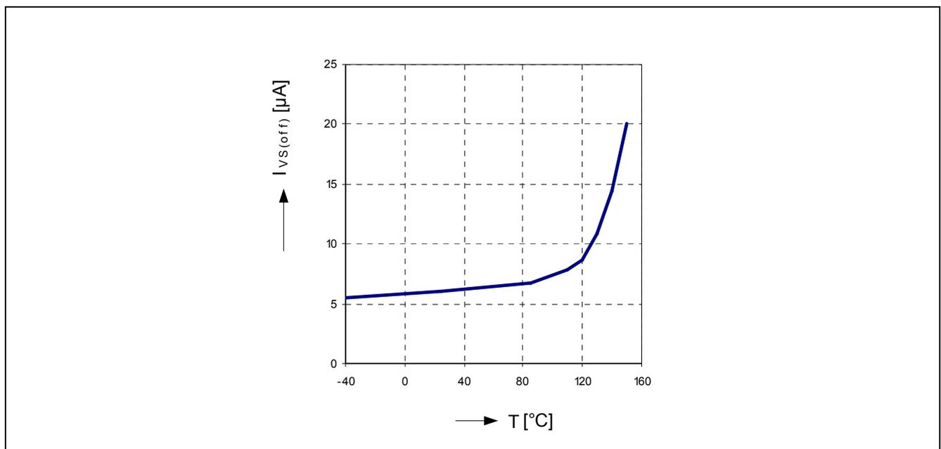
Figure 5 Typical Quiescent Current vs. Junction Temperature
