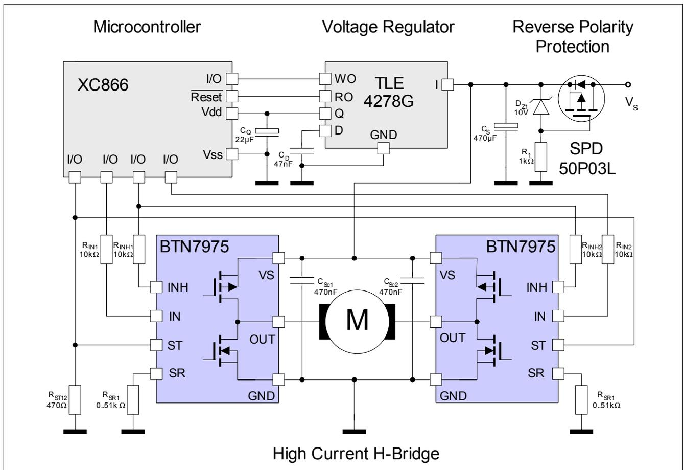
Figure 14 Application Example: H-Bridge with two BTN7975B
