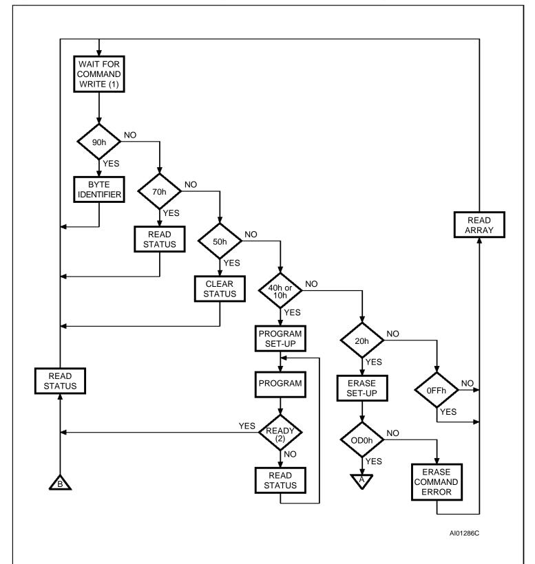
Figure 14. Command Interface and Program Erase Controller Flow-diagram (a)
