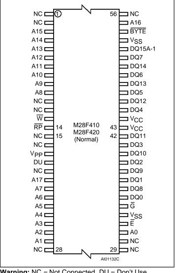
Figure 2B. SO Pin Connections
