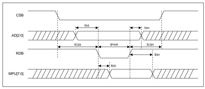
'Read(1)' means microcontroller reads MPU[7:0] CSB should keep 'High' to read.
