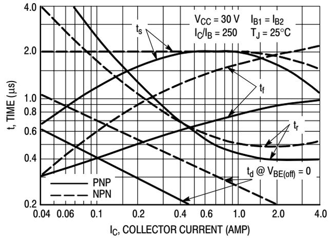
**Figure 2. Switching Times**
