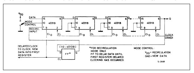
CASCADING USING HALF CLOCK PULSE DELAYED DATA OUTPUT (Q') TO PERMIT USE OF SLOW RISE AND FALL TIME CLOCK INPUTS
