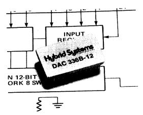
At the heart of the DAC336-12 is a laser-trimmed, low drift, thin-film nichrome network. The units accept TTL/ DTL and 5V CMOS logic levels and deliver a minimum of 5 mA at  $\pm$  10V out. Simple pin jumpering allows the user output choices of either  $\pm$  10V or 0 to  $\pm$  10V.
