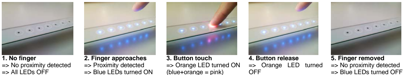
Figure 63 Touch+Proximity Module Operation
