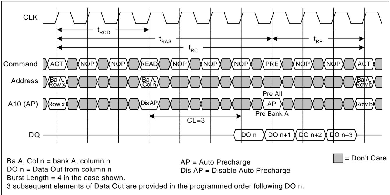
**Figure 14 Single READ Burst (CAS Latency = 3)**
