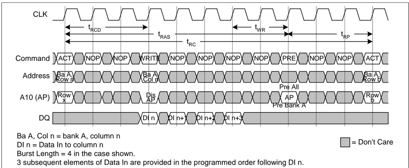
**Figure 26 WRITE Burst (CAS Latency = 3)**
