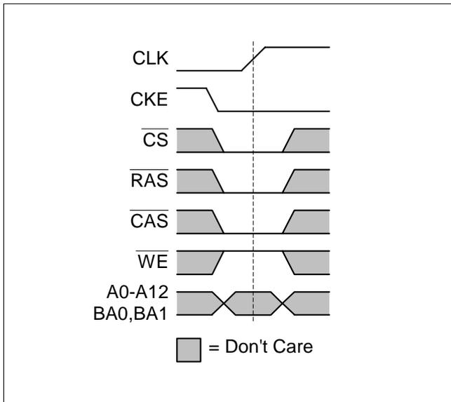
The SELF REFRESH command can be used to retain data in the Mobile-RAM, even if the rest of the system is powered down. When in the self refresh mode, the Mobile-RAM retains data without external clocking. The SELF REFRESH command is initiated like an AUTO REFRESH command except CKE is LOW. Input signals except CKE are “Don’t Care” during SELF REFRESH.
