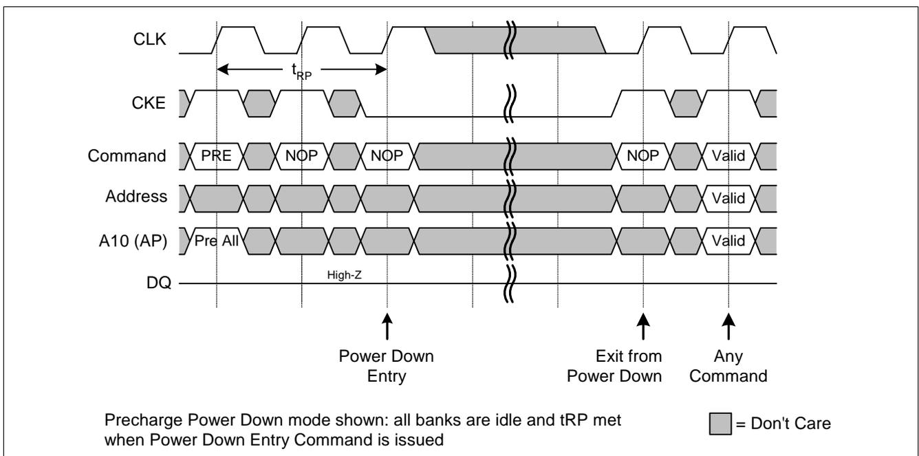
Figure 46 Power Down Entry and Exit
