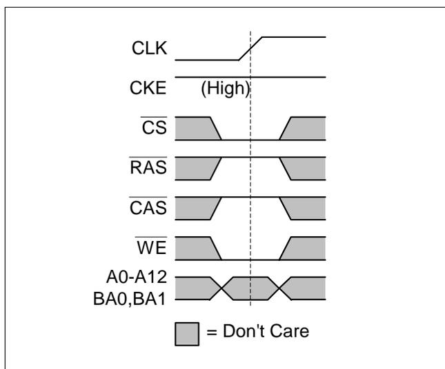
Figure 35 BURST TERMINATE Command
