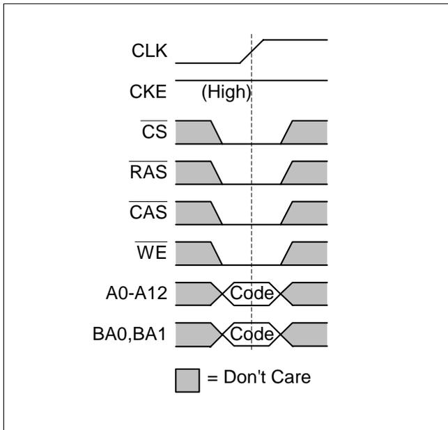
The Mode Register and Extended Mode Register are loaded via inputs A0 - A12 (see mode register descriptions in [Chapter 2.2](#)). The MODE REGISTER SET command can only be issued when all banks are idle and no bursts are in progress. A subsequent executable command cannot be issued until  $t_{MRD}$  is met.
