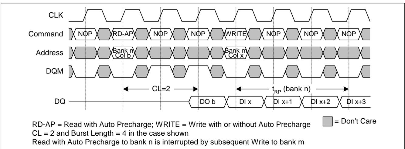
**Figure 38 READ with Auto Precharge Interrupted by WRITE**
