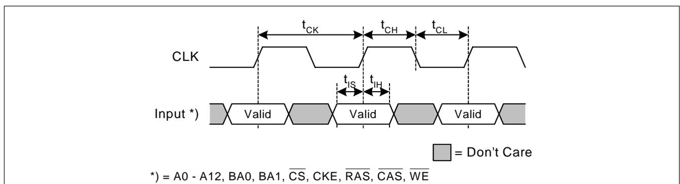
**Figure 5 Address / Command Inputs Timing Parameters**
