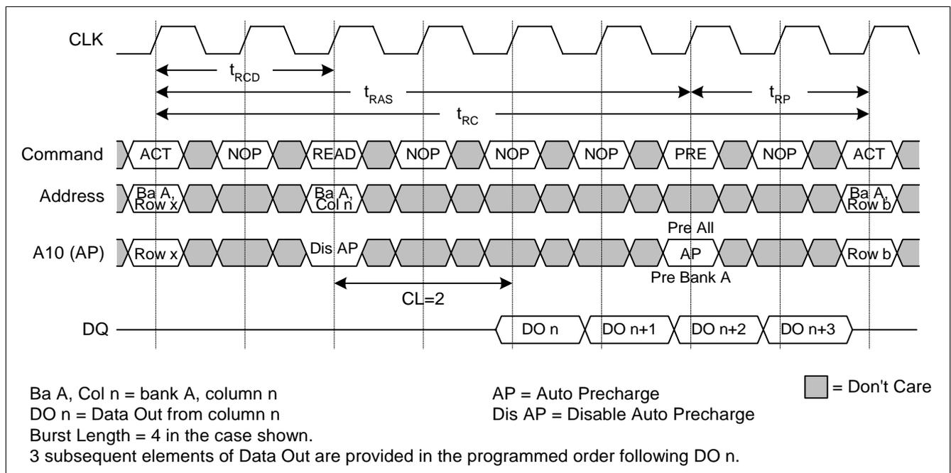
**Figure 13 Single READ Burst (CAS Latency = 2)**
