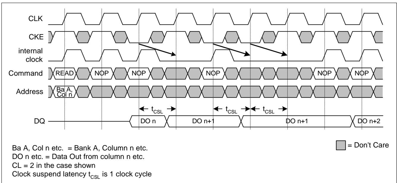
**Figure 19 Clock Suspend Mode for READ Bursts**
