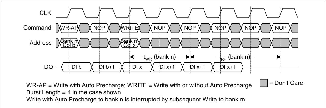
Figure 40 WRITE with Auto Precharge Interrupted by WRITE
