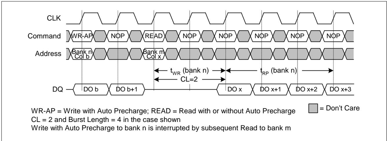
Figure 39 WRITE with Auto Precharge Interrupted by READ
