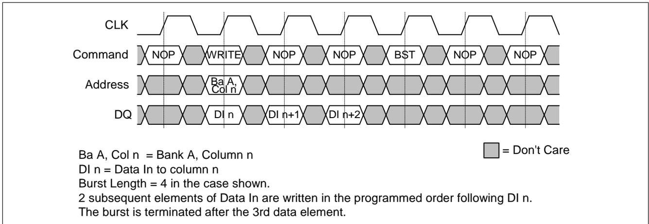
Figure 30 Terminating a WRITE Burst
