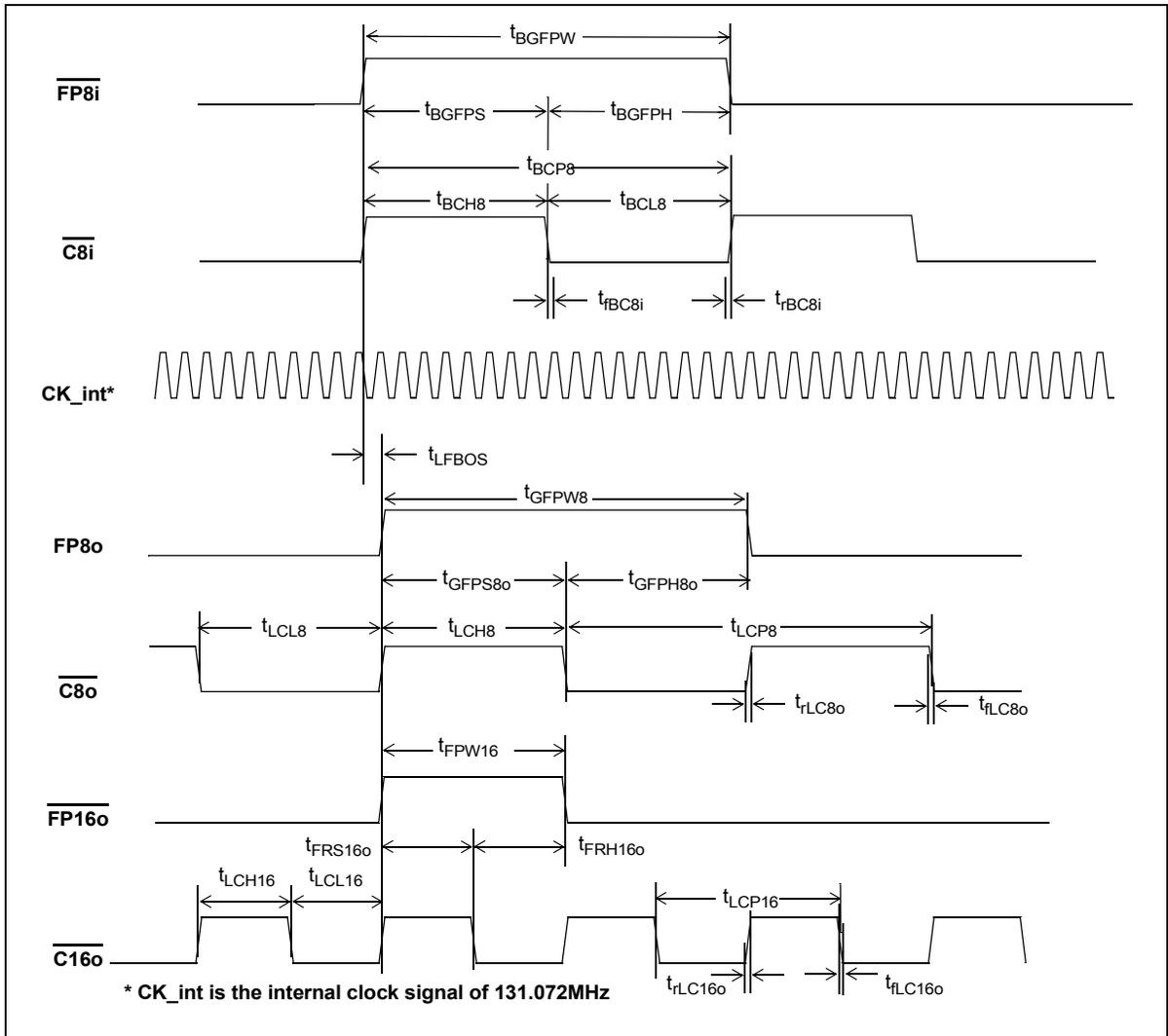
Figure 21 - Backplane and Local Clock Timing for GCI-BUS
