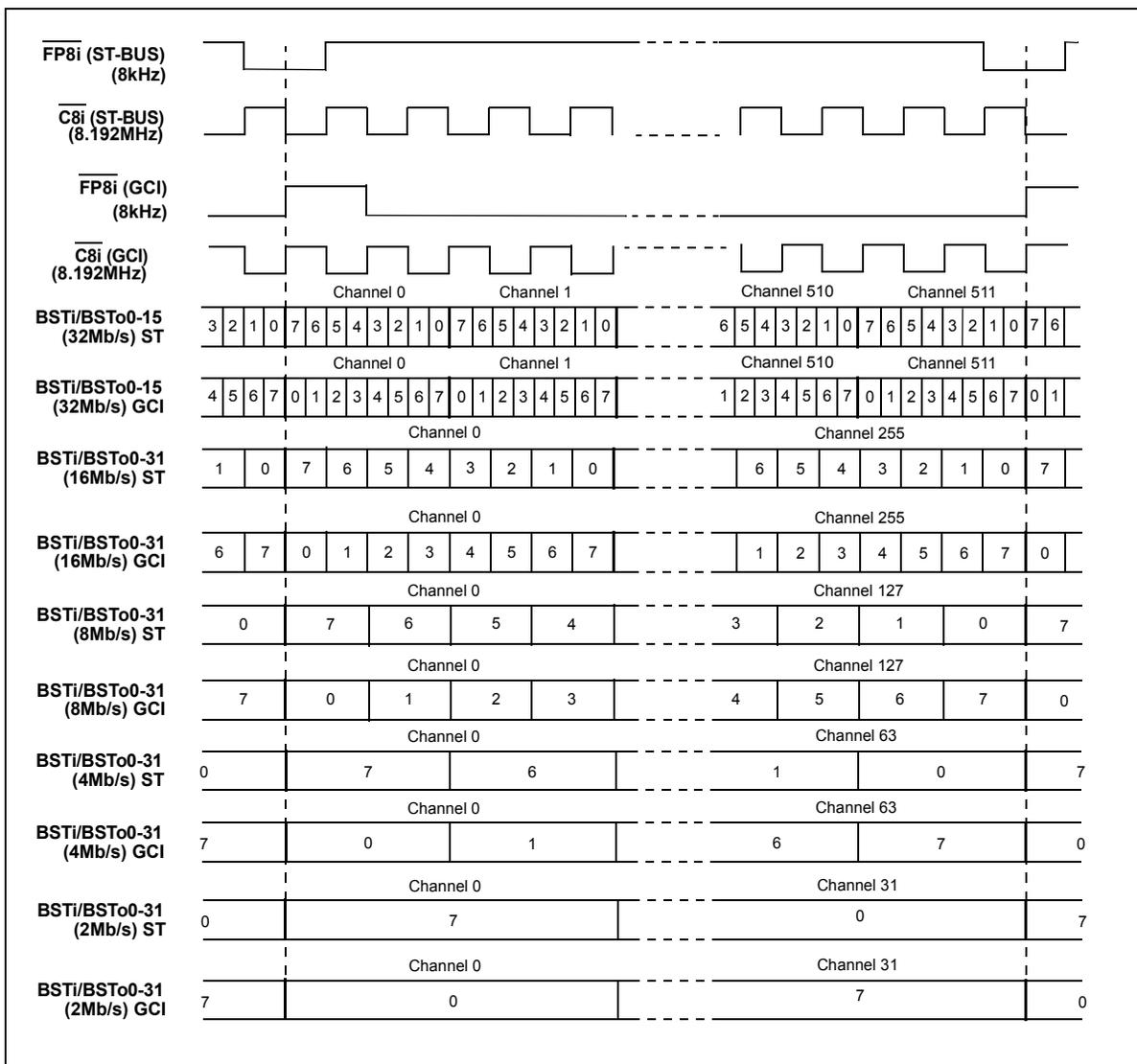
Figure 7 - Backplane Port Timing Diagram for 2, 4, 8, 16 and 32Mb/s stream rates
