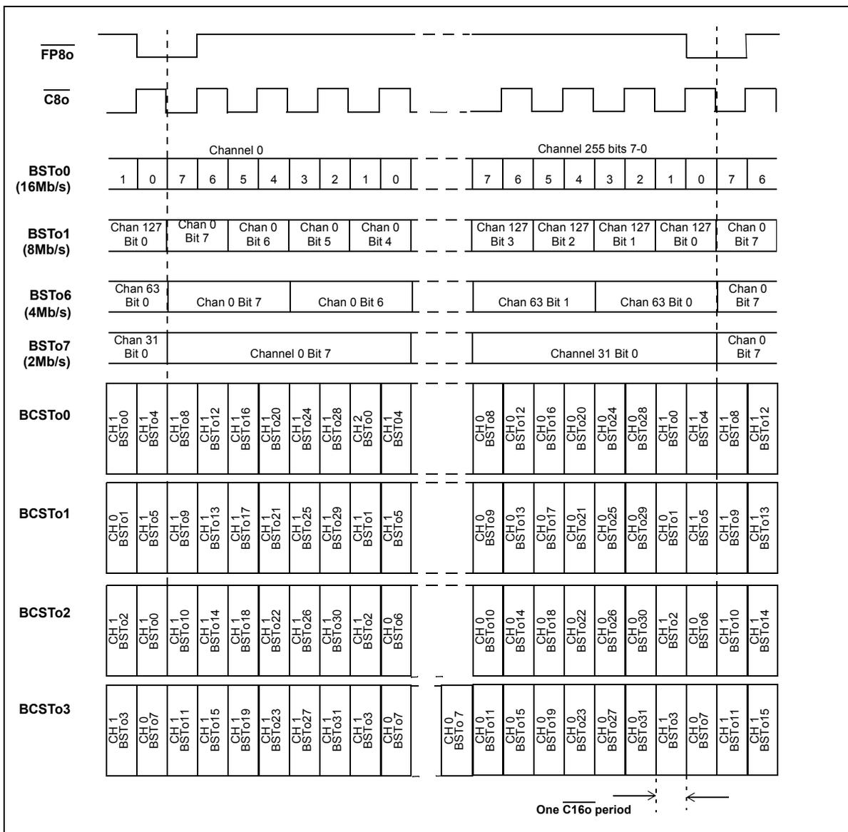
Figure 14 - Backplane Port External High Impedance Control Bit Timing (Non-32Mb/s mode)
