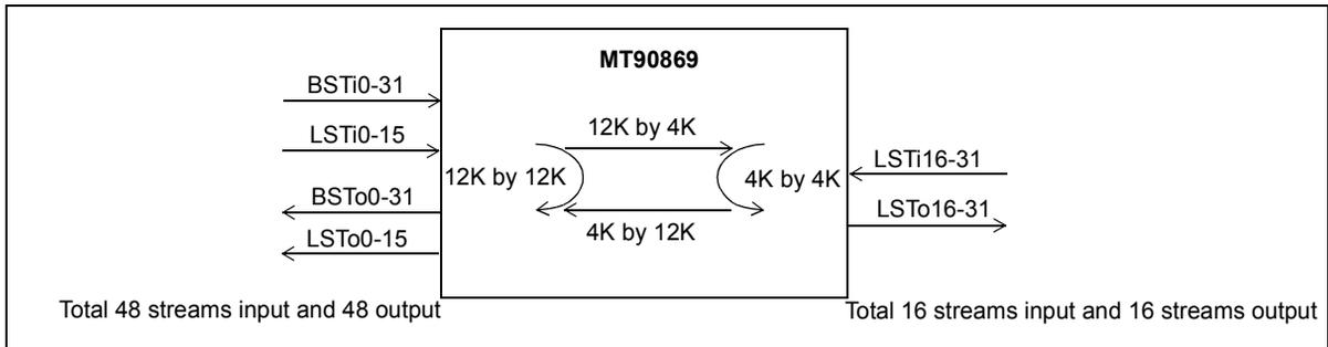
Figure 5 - 12K by 4K Blocking Configuration
