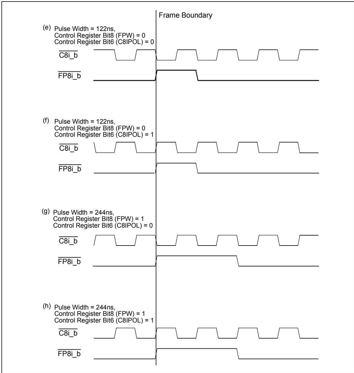
Figure 19 - Frame Boundary Conditions, GCI - BUS Operation
