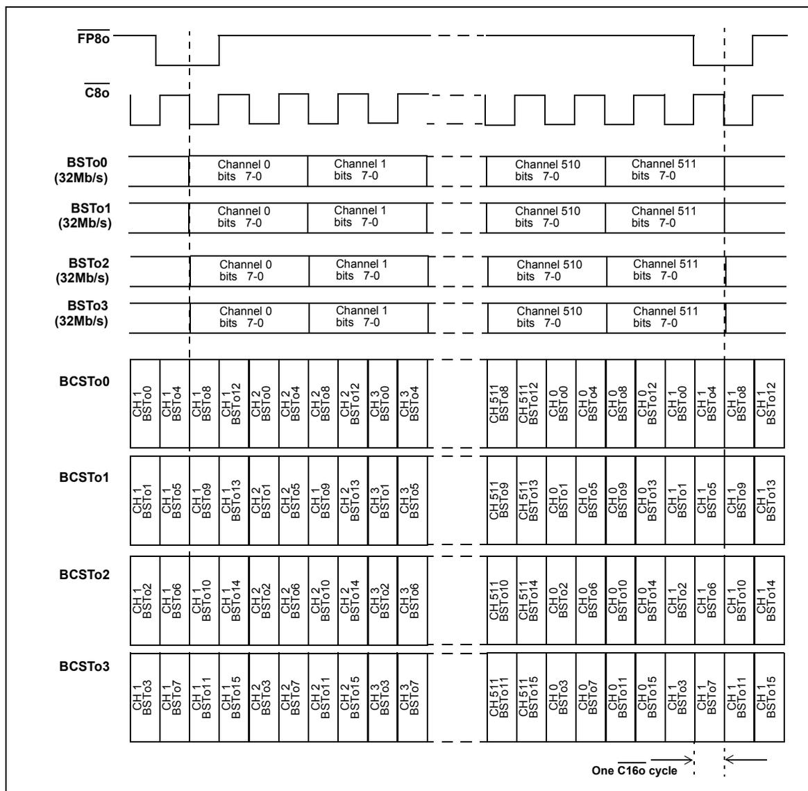
Figure 15 - Backplane Port External High Impedance Control Timing (32Mb/s Mode)
