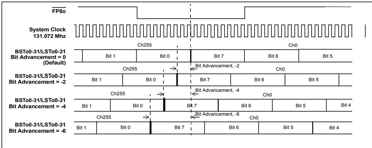
Figure 12 - Backplane and Local Output Advancement Timing diagram for Data Rate of 16Mb/s
