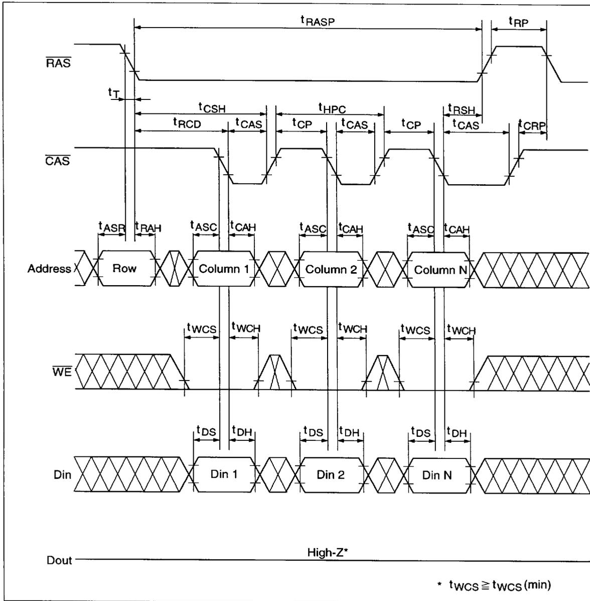
EDO Page Mode Delayed Write Cycle<sup>\*18</sup>
