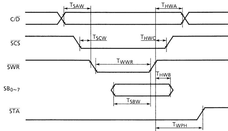
4.13 Timing Chart for Slave Bus Interface:  $\overline{DS}$ ,  $R/\overline{W}$  Bus Mode
