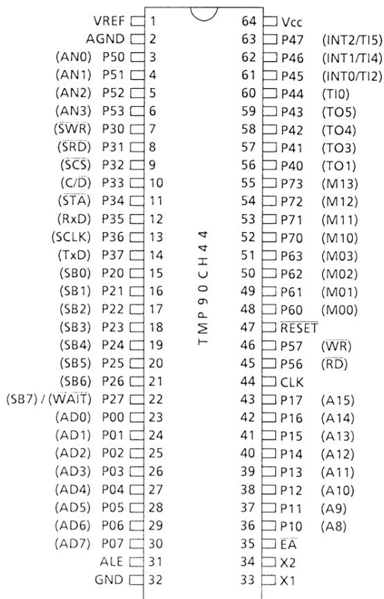
Figure 2.1 (1). Pin Assignment (Shrink DIP)
