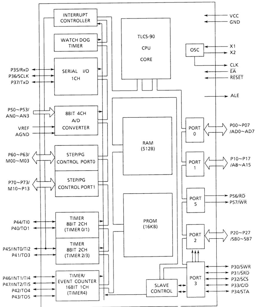
Figure 1. TMP90C844 Block Diagram
