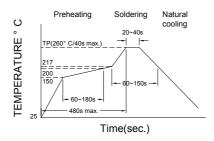
Figure 1. Re-flow Soldering
