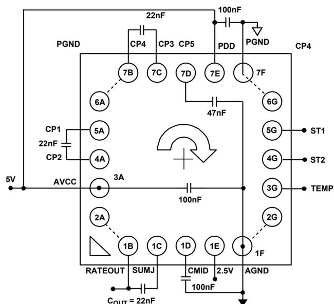
NOTE THAT INNER ROWS/COLUMNS OF PINS HAVE BEEN OMITTED FOR CLARITY BUT SHOULD BE CONNECTED IN THE APPLICATION.
