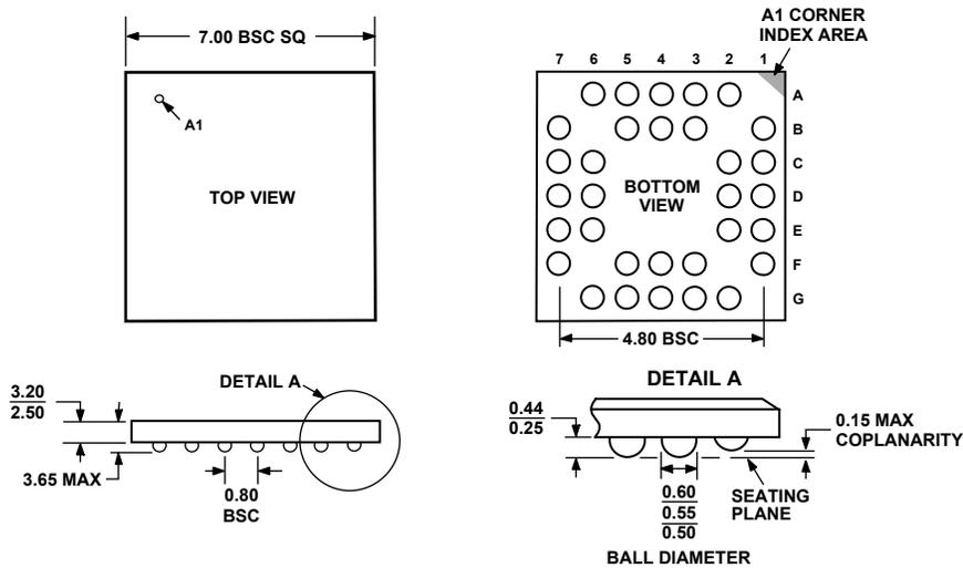
Figure 6. 32-Lead Chip Scale Ball Grid Array [CSPBGA]
