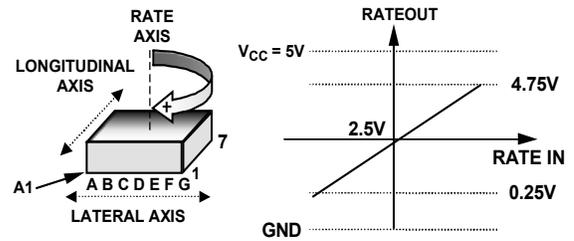
Figure 2. RATEOUT Signal Increases with Clockwise Rotation
