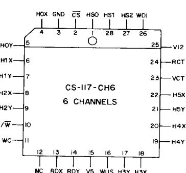
**ELECTRICAL CHARACTERISTICS:** V5=4.5 to 5.5V, V12=10.8 to 13.2V,
