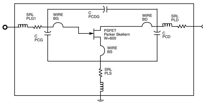
The PSFET is a Mimix implementation of the Parker Skellern large signal model. The model is available as an ADS project file on-line at: [www.mimixbroadband.com](http://www.mimixbroadband.com)
