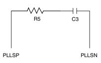
$\begin{array}{l} \textbf{SONET} \\ \textbf{R5} = 80 \Omega \\ \textbf{C3} = 1.5 \mu F \left( \text{X7R Dielectric} \right) \end{array}$
