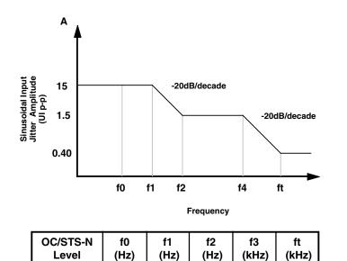
Figure 1. Input Jitter Tolerance
