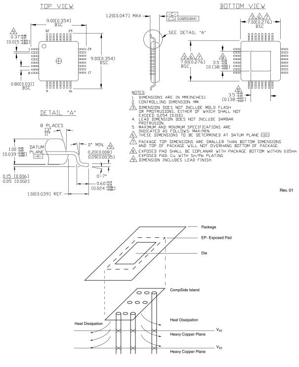
PCB Thermal Consideration for 32-Pin EPAD-TQFP Package
