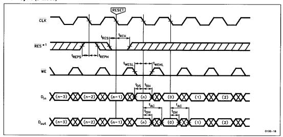
Note: \*1. The read address counter is reset at the first falling edge of  $\overline{\text{CLK}}$  after  $\overline{\text{RES}}$  falls, meeting the specifications of  $t_{\text{REPS}}$  and  $t_{\text{REPH}}$ , and it is not reset at the next falling edge of  $\overline{\text{CLK}}$  even if  $\overline{\text{RES}}$  is kept low.
