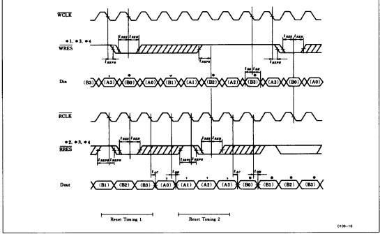
Notes: \*1. The write address counter is reset at the first falling edge of WCLK after WRES falls, meeting the specifications of t<sub>REPS</sub> and t<sub>REPH</sub>, and it is not reset at the next falling edge of WCLK even if WRES is kept low.
