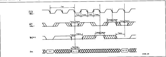
Note: \*1. When twTsL, twTHL, twEHL, and twEHH cannot meet the specifications, the write enbable operation is not guaranteed.
