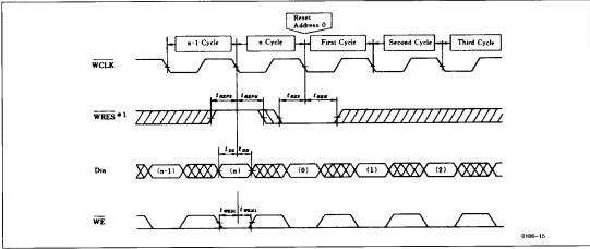
Note: The write address counter is reset at the first falling edge of WCLK after WRES falls, meeting the specifications of t<sub>REPS</sub> and t<sub>REPH</sub>, and it is not reset at the next falling edge of WCLK even if WRES is kept low.
