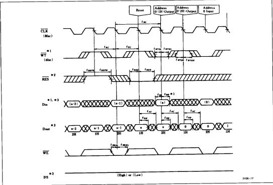
Notes: \*1. WT is the input during half cycle of CLK, meeting the specifications of twtsl, twthl, twtsh, and twthl. Data is written when WT is low. Reset is possible when WT is high.
