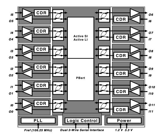
The **BCM8426** is an intelligent back end loop circuit that facilitates the implementation of an IBOD (Intelligent Bunch of Disks) on Fibre Channel Storage Array Systems. The **BCM8426** has an integrated EyeOpener<sup>®</sup> designed on-chip to drive optical and copper ports in fibre channel applications.
