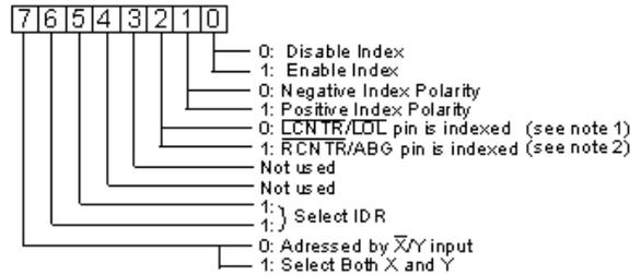
**Note 1:**  $\overline{\text{LCNTR/LOL}}$  input must also be initialized as the Load CNTR or the Load OL input via the IOR register bit 1.
