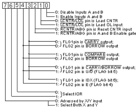
Control functions may be combined. The toggle flip flops are triggered by the trailing edges of the associated Carry, Borrow, or Compare match. Thus there is a 1-clock delay between the input and output of each flip flop. Unless otherwise specified, assume the longest prop delay from any input to any output is <110ns.
