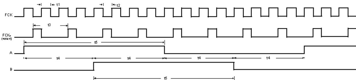
**Note 4:** FCKn is the final modulo-n internal filter clock, arbitrarily shown here as modulo-1.
