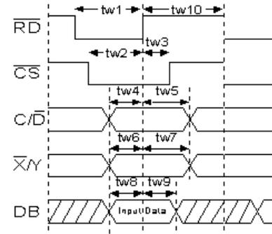
**Read Cycle Timing:** The data bus will become valid 50ns after asserting both Read and Chip Select. Release starts when either Read or Chip Select is terminated.
