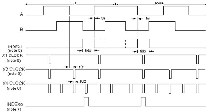
**Note 5 :** Shown here is positive index with solid line depicting 1/4 cycle index and dotted line depicting 1/2 cycle index. Either LCNTR/LOL or RCNTR/ABG input can be used as the INDEX input.
