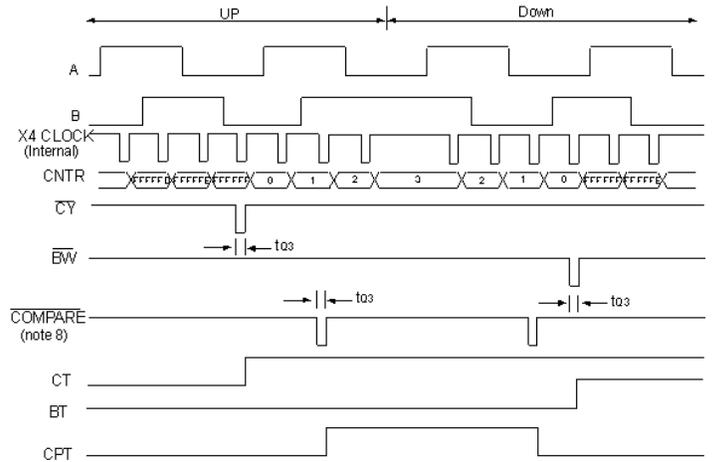
**Note 8 :** COMPARE is generated when PR = CNTR. In this timing diagram it is arbitrarily assumed that PR = 1.
