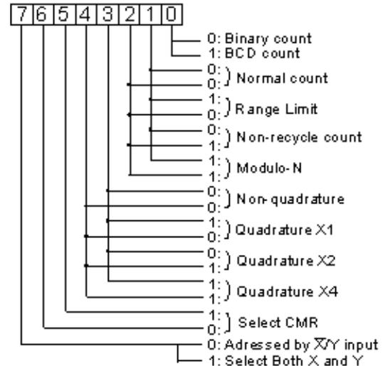
**Range Limit:** In range limit count mode, an upper and a lower limit is set, mimicking limit switches in the mechanical counterpart. The upper limit is set by the content of the PR and the lower limit is set to be 0. The CNTR freezes as  $CNTR = PR$  when counting up and at  $CNTR = 0$  when counting down. At either of these limits, the counting is resumed only when the count direction is reversed.
